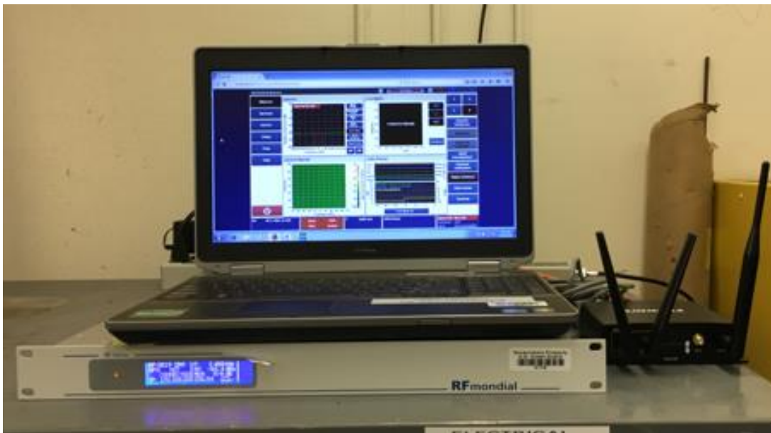
Figure 7. Alaska field test receive installation (Laptop and DRM Receiver).
