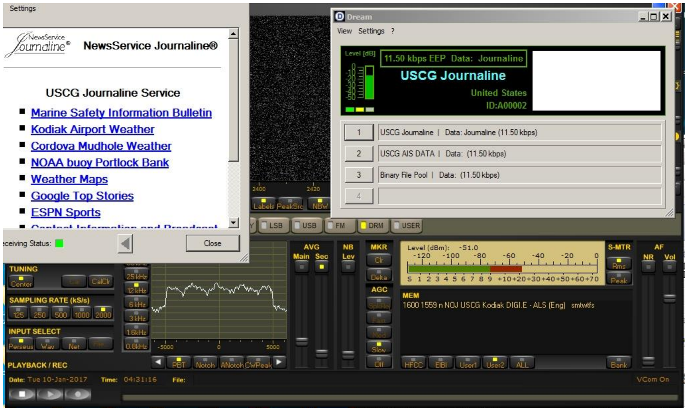
Figure 2. The end user reads the USCG Journaline service as if it was a web page.
