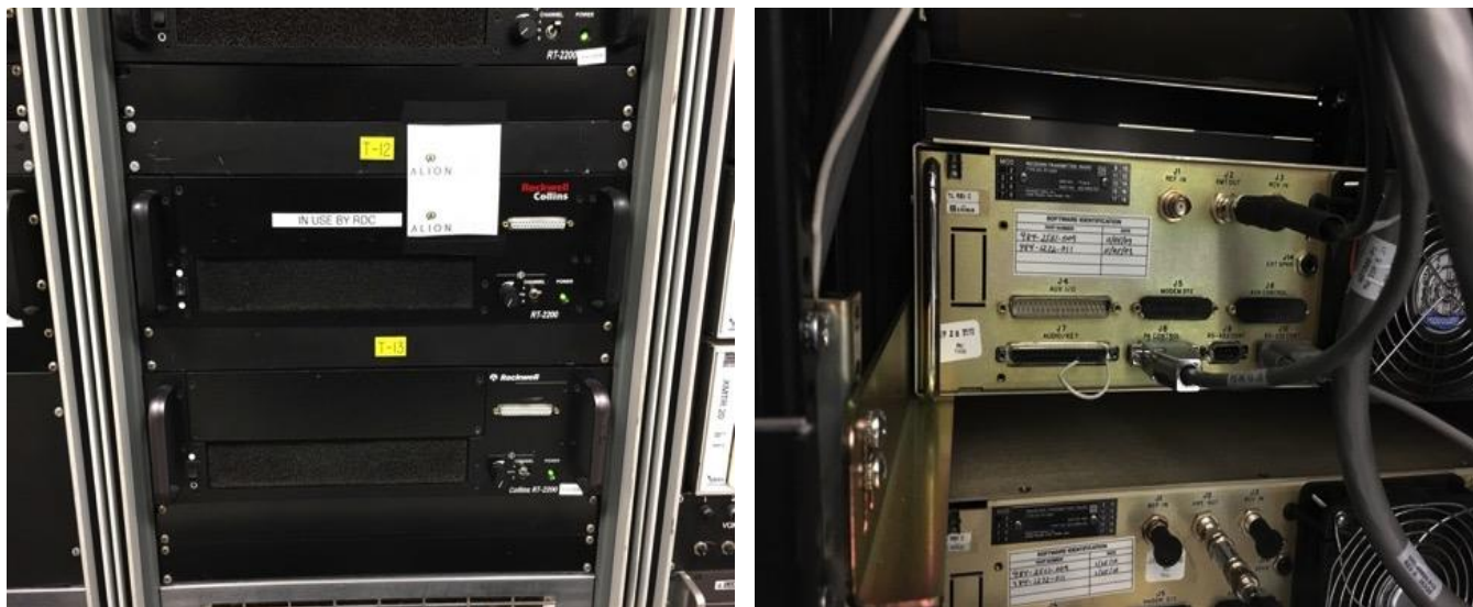
Figure B-4. Front of Rockwell Collins RT-2200 Exciter (left), rear of RT-2200 showing jumper location (right).
