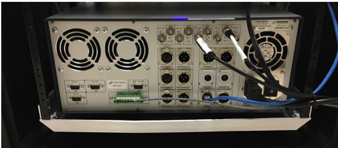
Figure B-6. Back of DMOD3 showing RF output and RF input connections.
