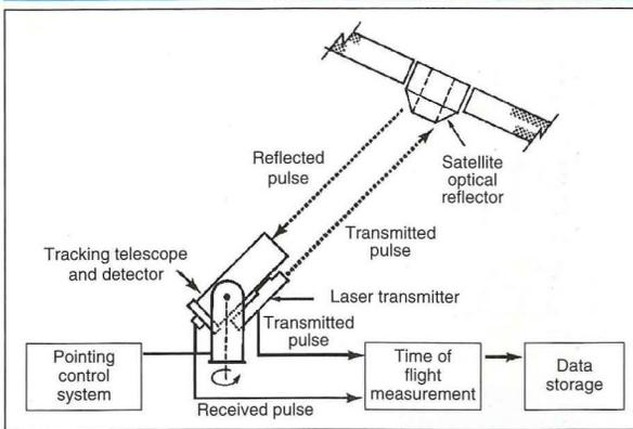
**Figure 1.** A simplified block diagram of a typical satellite laser ranging (SLR) station. By measuring the elapsed time between the transmission of a laser pulse and the reception of the pulse reflected by the satellite, the range to the satellite can be determined.
