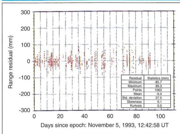
**Figure 5.** Range residuals from a fit of SLR data to a 104-day orbital arc for GPS-35
