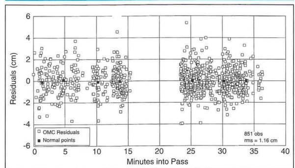
**Figure 4.** Range residuals from the analysis of data from a pass of GPS-35 collected by the MOBLAS-4 system at Quincy, California, on March 9, 1994, starting at 03:47 UT.
