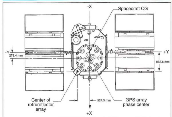
**Figure 3.** A sketch of a GPS satellite shows the locations of the retroreflector array, antenna array phase center, and the satellite center of gravity (CG). The positive Z-direction points out of the page.
