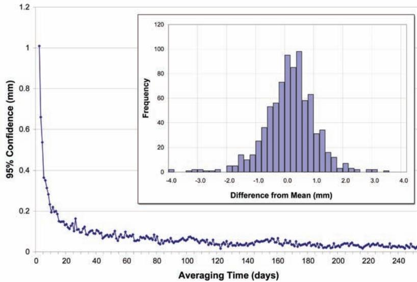
▲ **FIGURE 8** Accuracy versus averaging time for LREF-ML35, with inset histogram
