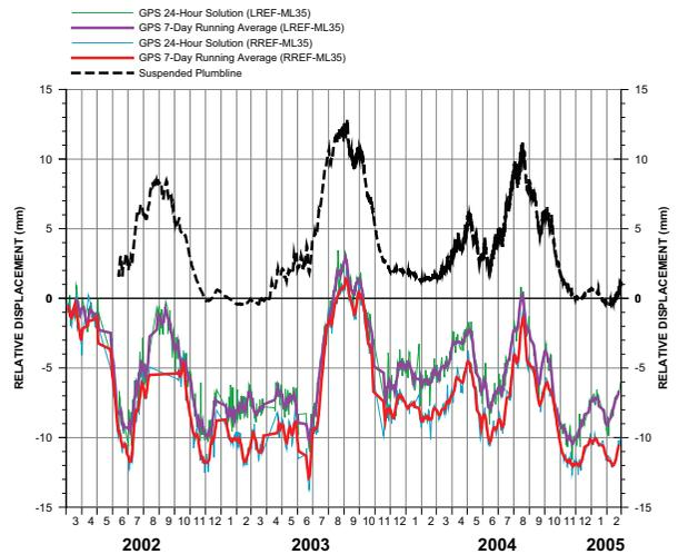
▲ FIGURE 3 Upstream-downstream displacement at ML35, plumb line, LREF GPS, and RREF GPS
