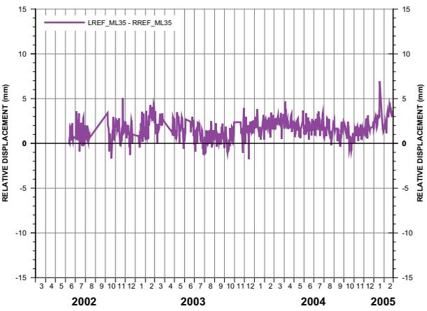
▲ FIGURE 5 Relative displacement between LREF GPS and RREF GPS at ML35
