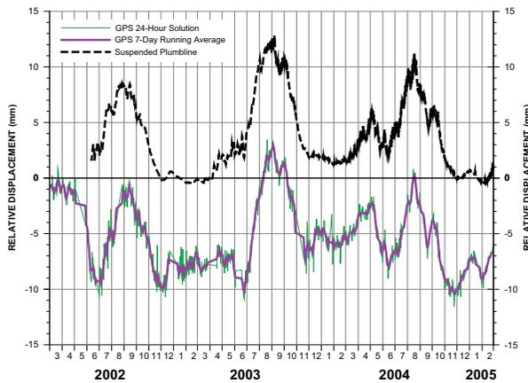
▲ FIGURE 2 Upstream-downstream displacement at ML35, plumb line and GPS (LREF)
