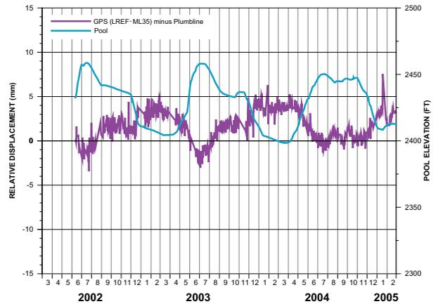
▲ **FIGURE 7** Bias between ML35 plumb line and ML35 GPS (LREF) plus pool elevation
