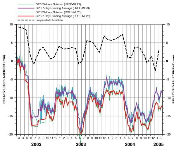
▲ FIGURE 4 Upstream-downstream displacement at ML23, plumb line, LREF GPS, and RREF GPS
