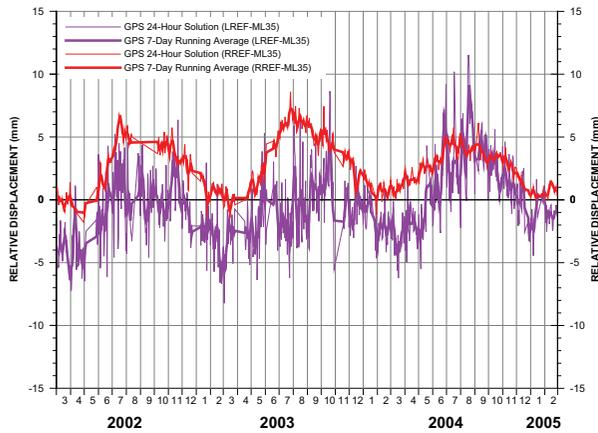
▲ **FIGURE 6** Vertical displacement at ML35, LREF GPS, and RREF GPS
