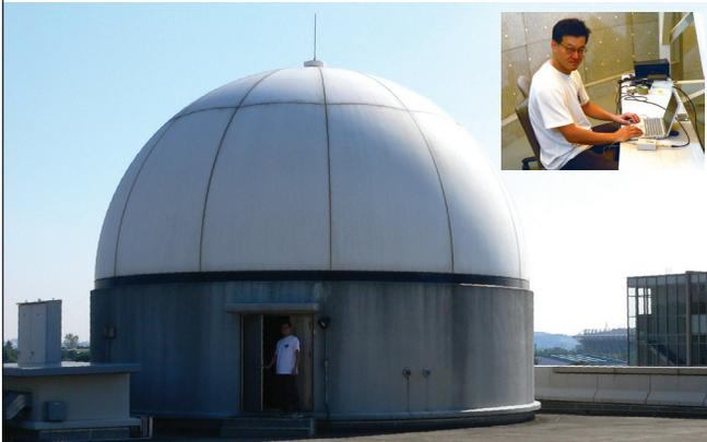
▲ **FIGURE 3** Toshiaki Tsujii stands in front of JAXA's radio-transparent dome test facility and (inset) is shown conducting a test on an iPRx receiver. The box to the right of the laptop contains the iPRx receiver hardware, with an embedded front-end module and USB interface.
