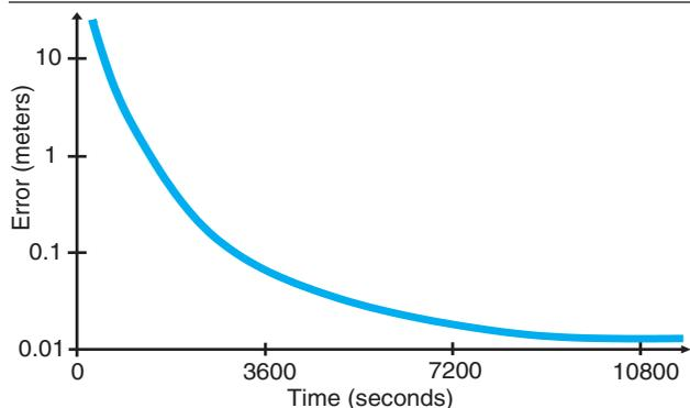
▲ **FIGURE 6** The approximate relationship between achievable accuracy of standalone positioning and the time required to achieve such accuracy. The regions where the plot converges to the axes represent the biggest challenges.
