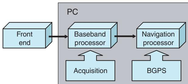
▲ **FIGURE 1** A block diagram of a PC-based snapshot software receiver, which has been developed to facilitate BGPS technology development and serves as a prototype for an airborne receiver. There are extra tracking loops for the airborne receiver, which are not shown here.
