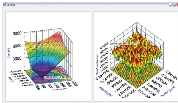
▲ **FIGURE 2** Example of a cost function, which has been plotted for the AGPS type of algorithm (left) and the BGPS type of algorithm (right). The AGPS solution allows one to put tight constraints on initial time and position assumptions. These figures are screenshots from the first version of our receiver, which was not able to find a position in real time due to the complexity of the cost function.
