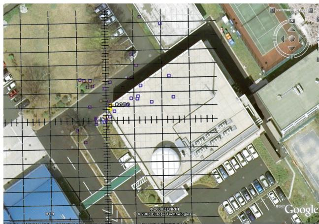
▲ **FIGURE 5** The output from an iPRx receiver passed to Google Earth. Each large division on the horizontal axis is 10 meters; on the vertical axis, 5 meters. The antenna used for this test is located on top of the JAXA building. A yellow pin depicts the true position of the antenna. Another test was conducted inside the radio-transparent dome, which can be seen in another corner of this building as a large circle.
