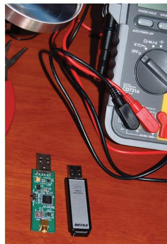
▲ **FIGURE 7** The USB stick-type front end for the iPRx receiver beside a standard USB memory stick.
