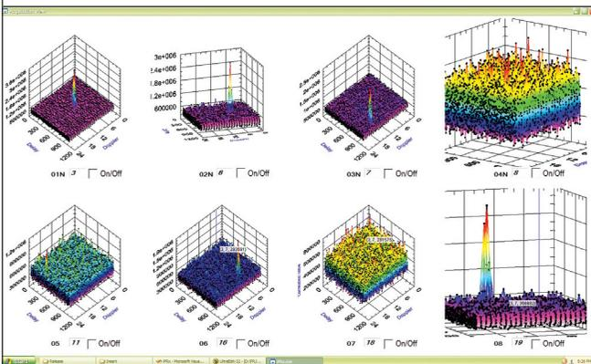
▲ **FIGURE 4** A screenshot of the iPRx software window showing acquisition selections. The horizontal axes represent code delay and Doppler shift. The plots are scalable and can be rotated to allow better visualization.
