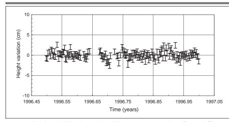
Figure 6. Height variability time series of Herstmonceux, southern England. The repeatability is 8 millimeters (derived with the best processing strategy).
