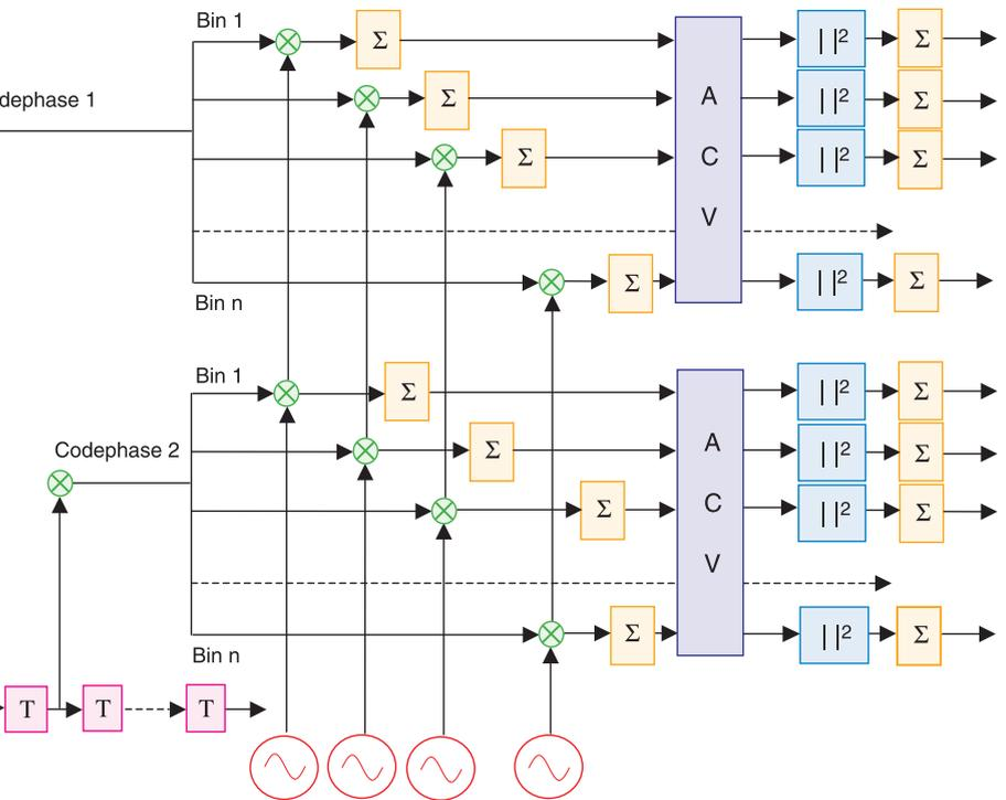
▲ **Figure 2** A two-code-phase subATTO search engine. In addition to the operational blocks described in Figure 1, the ACV (autoconvolution) block constitutes a proprietary algorithm utilizing multiple fast Fourier transform (FFT) bins. The FFT/ACV/squarer process provides improved sensitivity for the same overall integration period compared to the technique of Figure 1.
