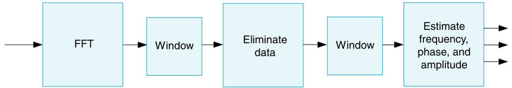
▲ **Figure 3** Core signal-processing scheme. The fast Fourier transform (FFT) block is equivalent to the ensemble of local oscillators, second mixers, and first summers of Figure 2, while the windowing and eliminate data blocks correspond to the ACV (autoconvolution) block in Figure 2. Various estimation algorithms are employed depending on the implementation.
