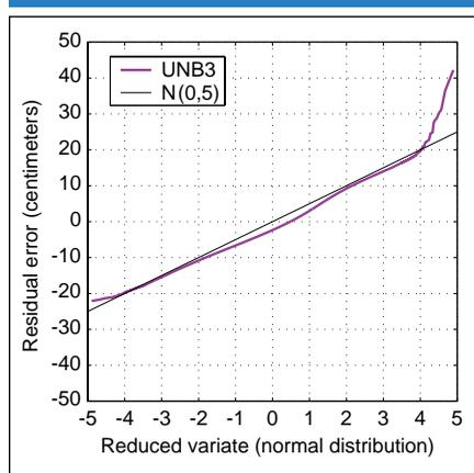
**Figure 3.** Gaussian plot of zenith delay residuals for UNB3. The thin line shows the zero-mean, 5-centimeter standard deviation normal distribution.
