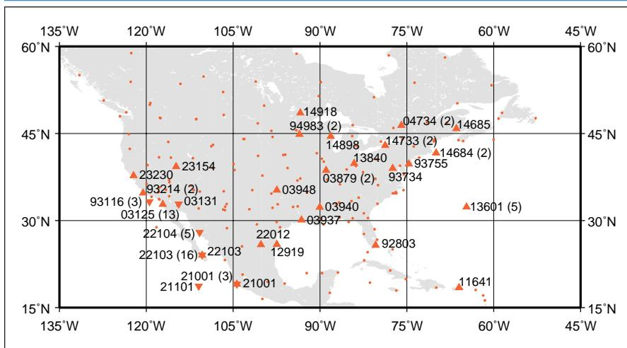
**Figure 4.** Location of radiosonde stations providing data between 1987 and 1996. In addition to their identification numbers, stations with positive extremes from model UNB3 are labeled ▲ and stations with negative extremes are labeled ▼. Parenthetical digits indicate the number of extremes for sites having more than one.
