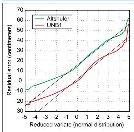
**Figure 2.** Gaussian plot of zenith delay residuals for the Altshuler model and UNB1. Thin lines represent best-fit normal distributions.
