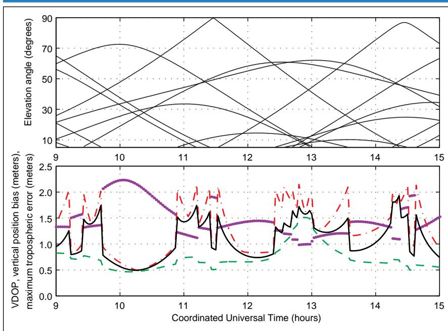
**Figure 6.** Satellite constellation at station 12919, Brownsville, Texas, on July 18, 1997, and simulated vertical position biases from a 21-centimeter zenith delay error. The solid and dashed lines show the unweighted and weighted solution biases respectively. The dashed and dotted line denotes maximum tropospheric error (the error at lowest elevation satellite), and the dotted line displays the vertical dilution of precision (VDOP).
