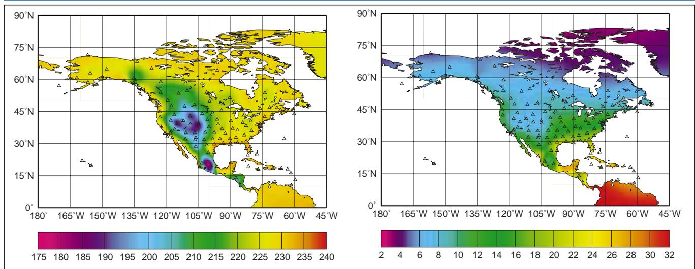
**Figure 1.** Mean hydrostatic (left) and wet (right) zenith delays in centimeters computed from radiosonde soundings made in 1992. Triangles indicate station locations.
