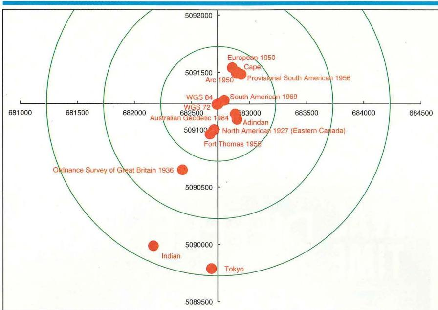
**Figure 1.** Using the wrong datum and associated ellipsoid when transforming and projecting latitudes and longitudes to map grid coordinates can result in large errors. This plot shows the corresponding UTM eastings and northings (in meters) of a point with WGS84 geographical coordinates of 45° 57' 0.96" N, 66° 38' 32.22" W, for a variety of geodetic datums. The circles have radii of 500, 1,000, and 1,500 meters.
