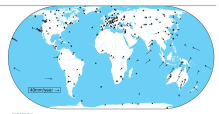
FIGURE 3 Calculated velocities of IGS stations from a recent weekly update of the IGS cumulative reference frame product. The velocities reflect the movement and deformation of the Earth's tectonic plates.
