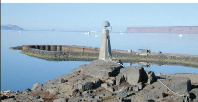
THE TAPER OF this pillar monument in Thule, Greenland, results in a top surface of smaller diameter than the antenna, which is recommended for pillar monuments.
