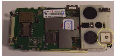
▲ FIGURE 5 Phone with GPS patch antenna at edge of PCB
