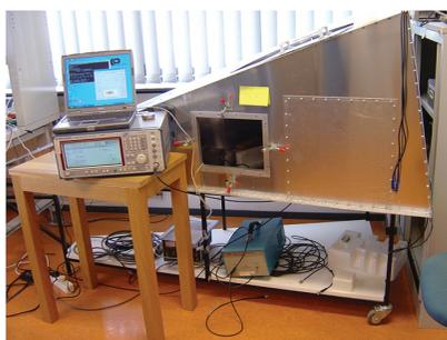
▲ **FIGURE 7** The GTEM cell and related test equipment
