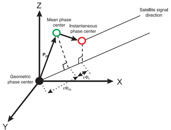
**▲ FIGURE 1** Geometry of GPS antenna phase center
