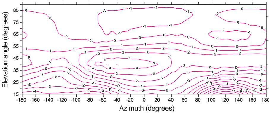
▲ **FIGURE 3** L1 phase-center variations (in millimeters) with respect to the relative mean phase center of conventional geodetic and choke-ring antennas resulting from the anechoic chamber calibration for an elevation mask angle of 15°
