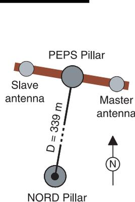
▲ FIGURE 2 Calibration beam installation
