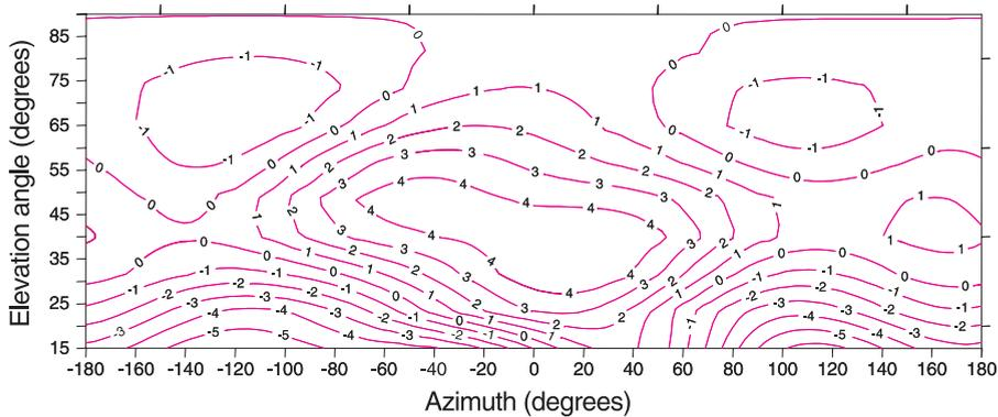
▲ **FIGURE 4** L1 phase-center variations (in millimeters) with respect to the relative mean phase center of conventional geodetic and choke-ring antennas resulting from the beam calibration (September 1995) and modeled with spherical harmonics ( $n=6, m=4$ ) for an elevation mask angle of 15°
