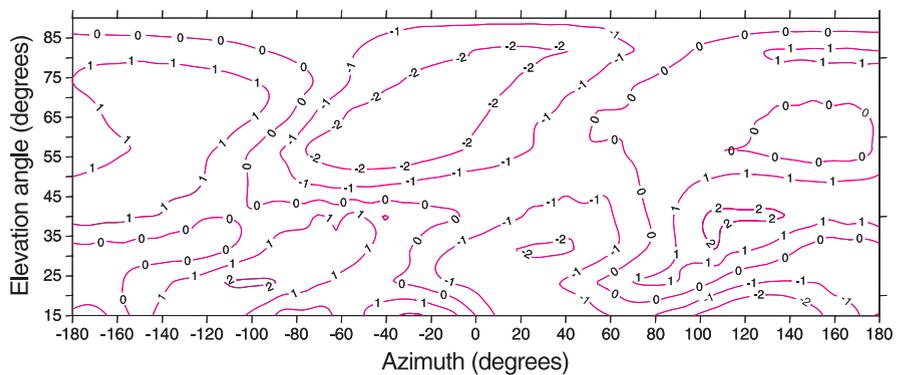
▲ **FIGURE 5** Difference (in millimeters) of the relative L1 phase-center variations resulting from the beam calibration and anechoic chamber techniques for an elevation mask angle of 15°
