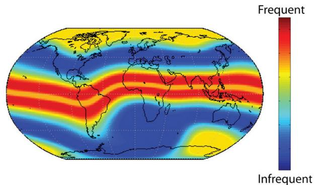
▲ **FIGURE 1** Global occurrence characteristics of scintillation. (Figure courtesy of P. Kintner)
