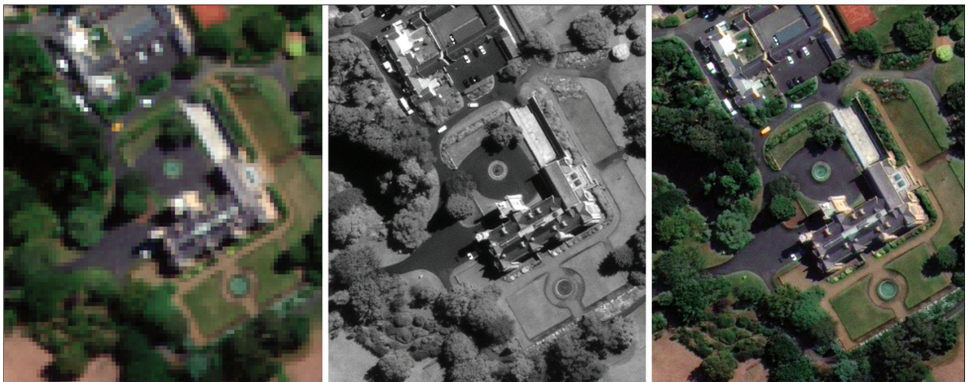
Figure 3: Fusion quality of UNB-Pansarp for GeoEye-1 images (launched in 2008). (a) Original GeoEye-1 MS image, 2m resolution; (b) Original GeoEye-1 Pan image, 0.5m; (c) Pan-sharpened GeoEye-1 MS image, 0.5m, using UNB-Pansarp.
