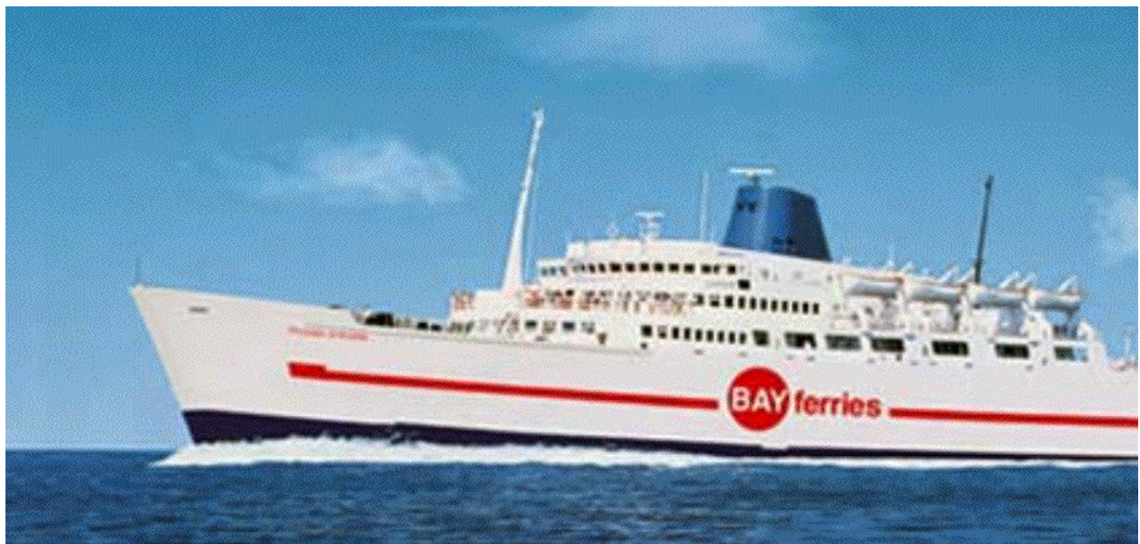
Figure 3. The Princess of Acadia. This car-ferry accommodates up to 650 passengers, 155 automobiles and 33 tractor-trailers. The ship was built in 1971, has a length of 146 m, beam of 20.5 m, and draft of 4.6 m.
