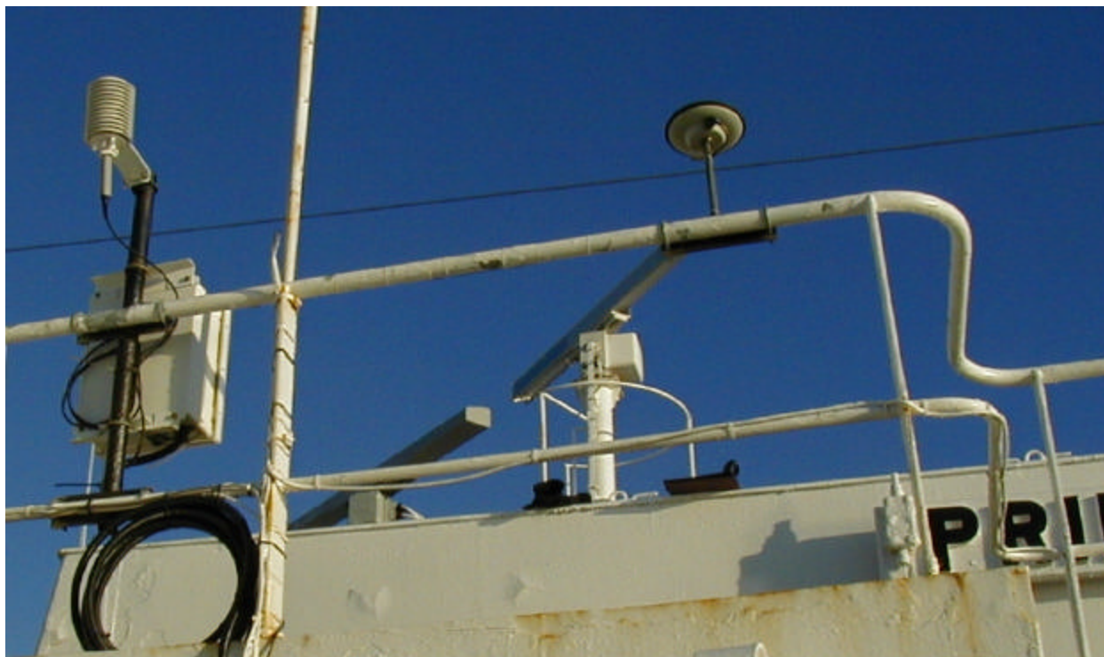
Figure 4. GPS and meteorological station locations on the Princess of Acadia. They are approximately 19 m above the vessel waterline.
