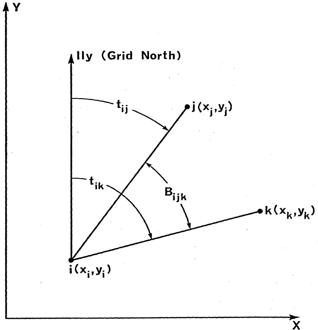
Figure 3.3 Angle on the Mapping Plane
