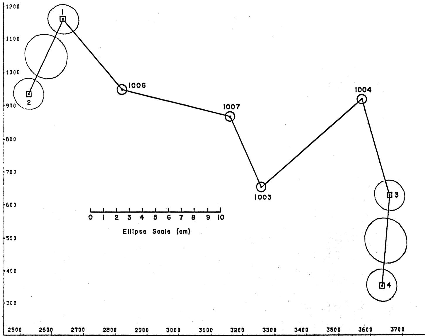
Figure 7.3 Initial Configuration for Closed Traverse with Weighted Points
