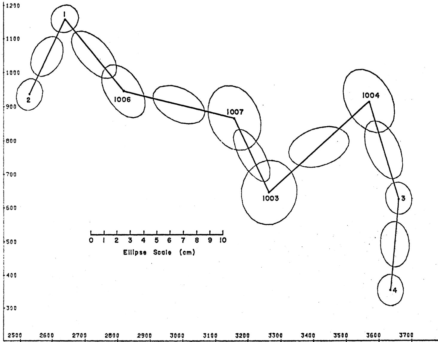
Figure 7.4 Plot of 95% Error Ellipses for Closed Traverse with Weighted Points
