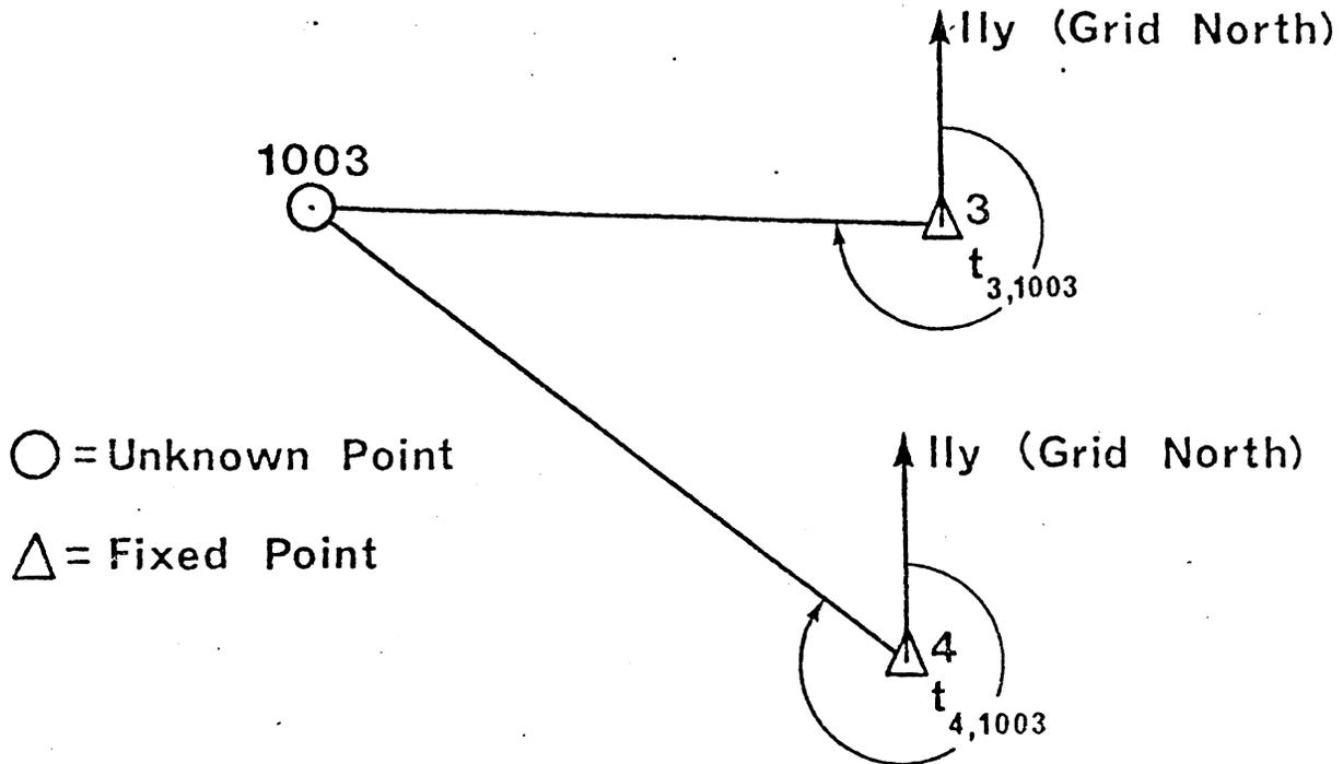
Figure 5.3 Azimuth Intersection on the Plane
