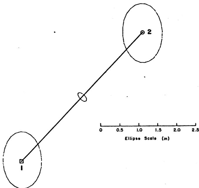
Figure 7.2 Plot of 95% Error Ellipses for Direct Case with Weighted Parameters
