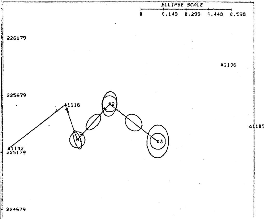
Figure 8.3 Plot of 99% Confidence Ellipses from Initial Observables.
