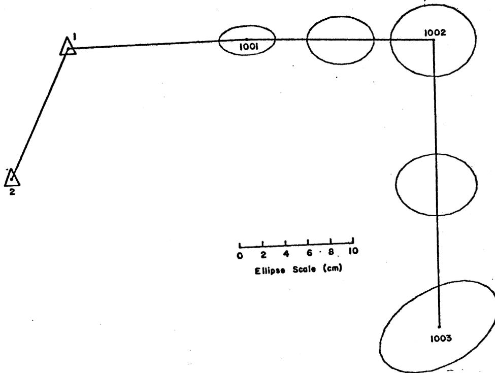
Figure 5.10 95% Confidence Ellipses for Open Traverse
