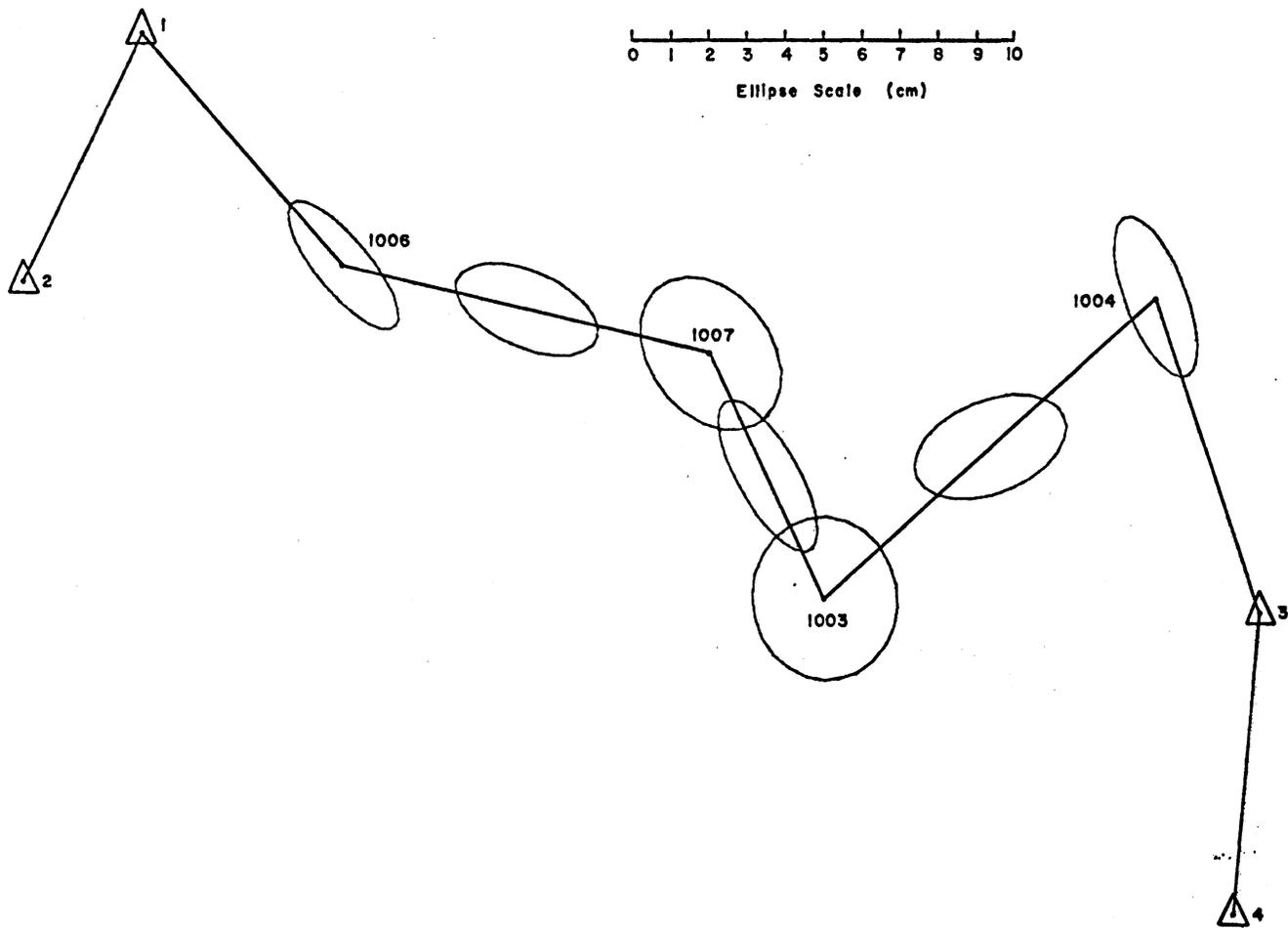
Figure 6.3 Plot of 95% Error Ellipses for Closed Traverse
