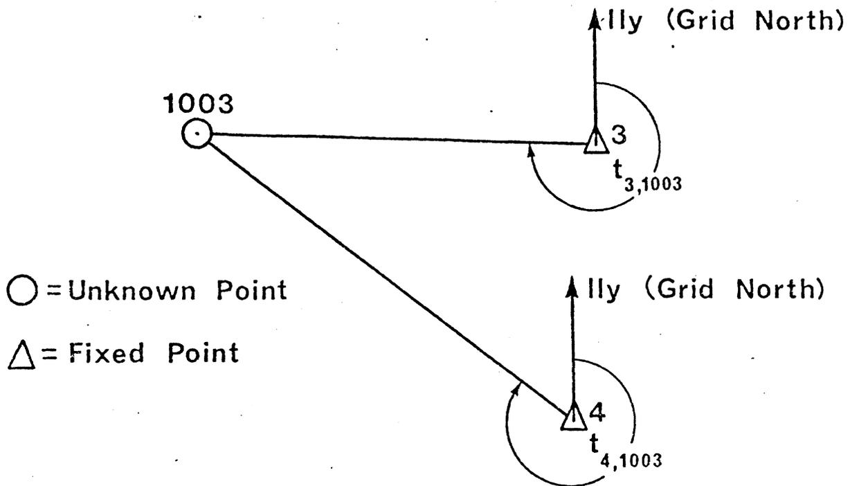
Figure 5.3 Azimuth Intersection on the Plane
