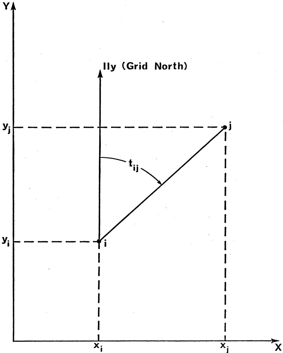
Figure 3.1 Mapping Plane Azimuth
