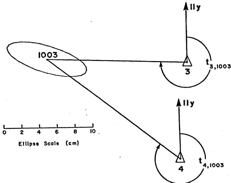
Figure 5.4 95% Confidence Ellipse for Azimuth Intersection
