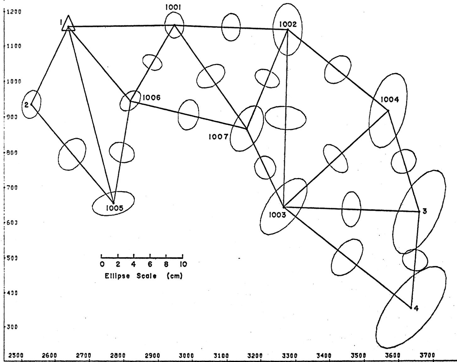
Figure 6.5 Plot of 95% Error Ellipses for the Network
