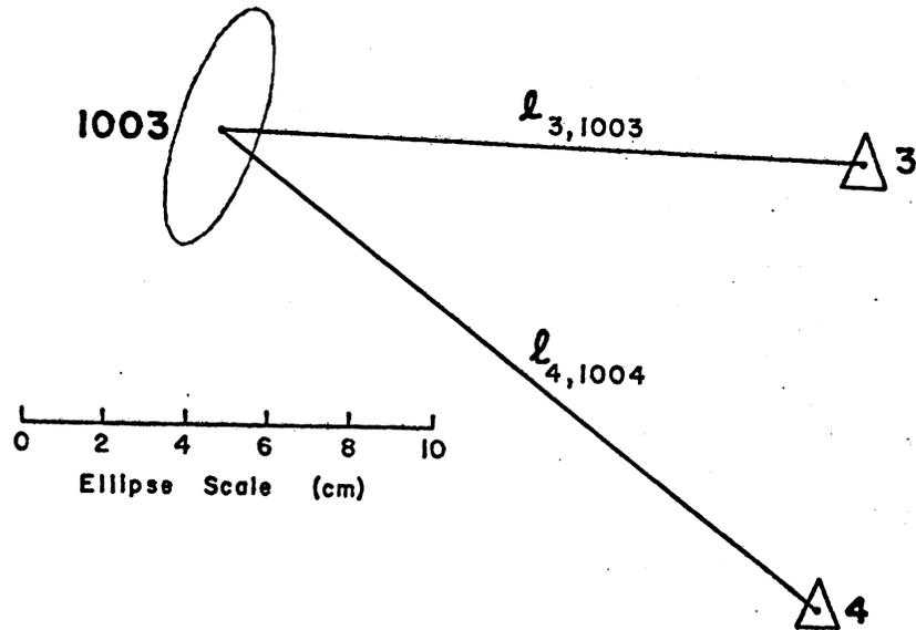
Figure 5.6 95% Confidence Ellipse for Distance Intersection
