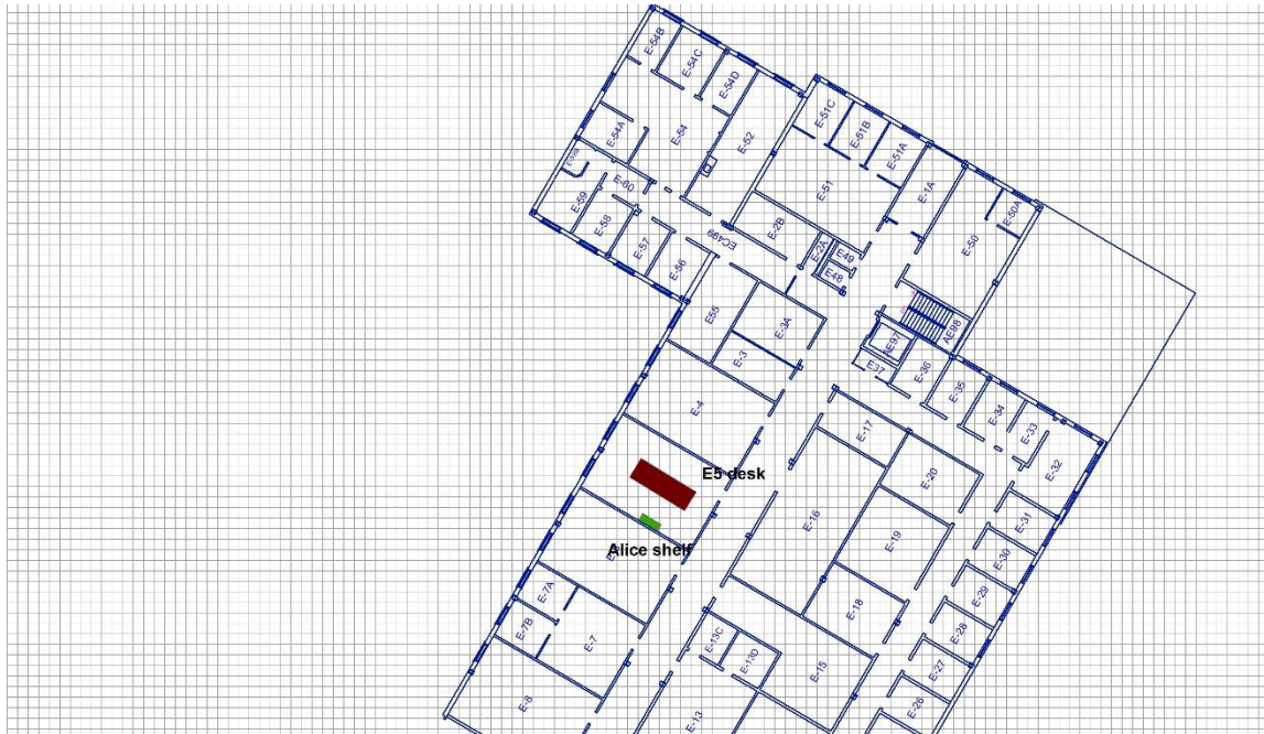
Figure 4.2 A grid of QTEM squares in resolution of 0.75-meter that covers Head Hall building and facilities
