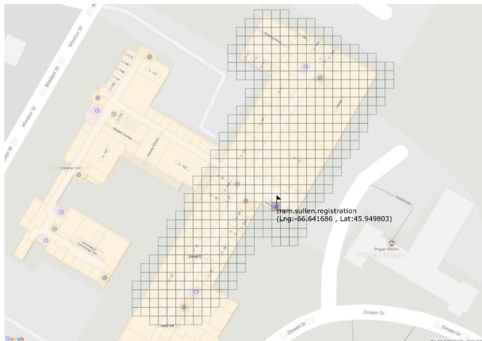
Figure 2.15 The original what3words grid over Head Hall complex. The annotated 3m x 3m square is used to encode the location of the main entrance
