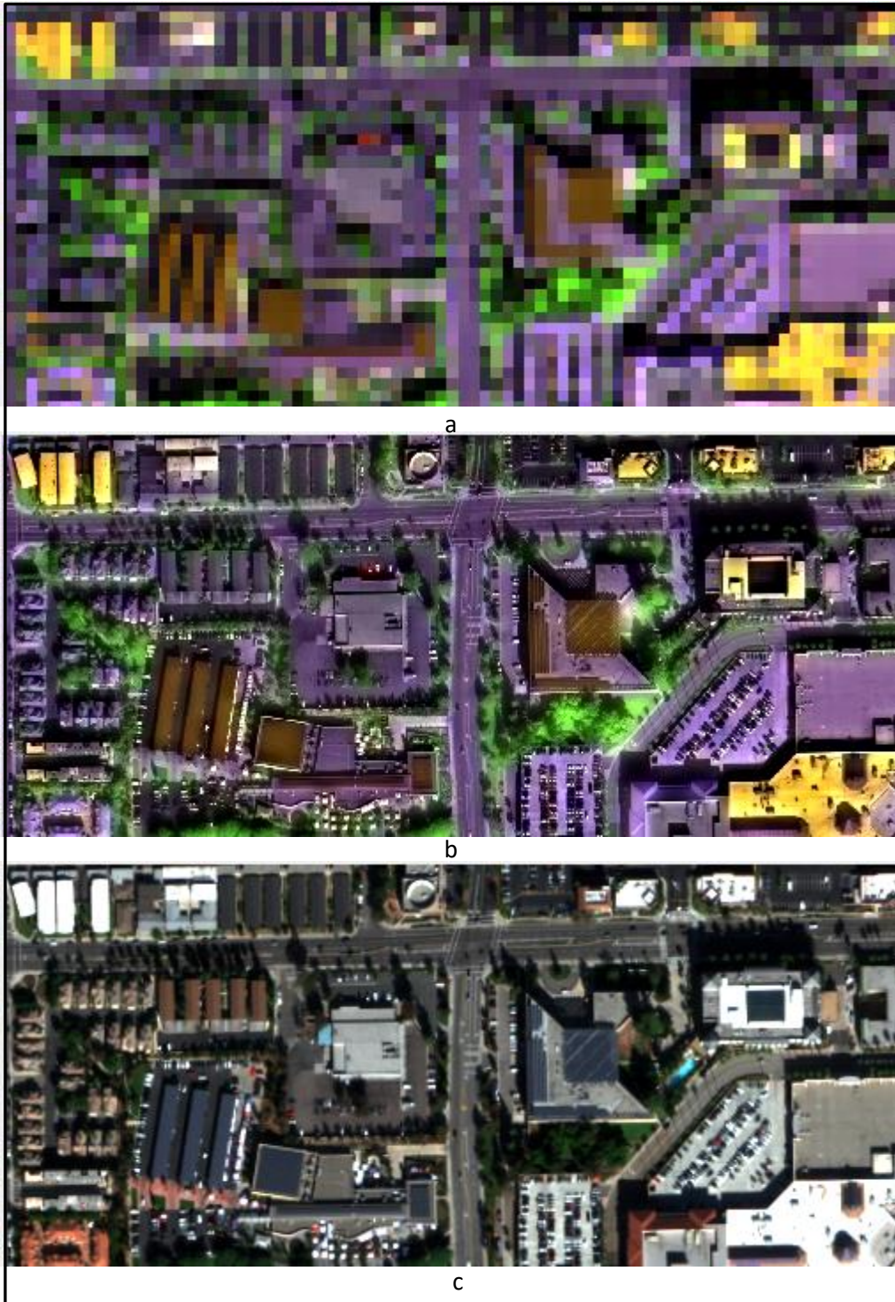
Figure 3.6 Comparison between the available 7.5m SWIR image (a), the 1.2m HR SWIR image generated using FGSS (b), and the original 1.2m VNIR image (c).
