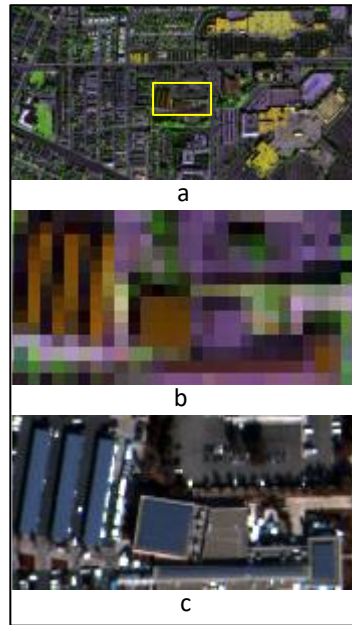
Figure 3.2 Solar PV panels in different spectral images of WorldView-3. (a) Available 7.5m SWIR bands 2, 1, 8 displayed in RGB at 1:1 ratio, (b) enlarged 7.5m SWIR bands, and (c) original 1.2m VNIR bands 5, 3, 2 displayed in RGB. (In the available SWIR bands small solar PV panel installations are not visible; however, they are clearly visible in the original VNIR bands.)
