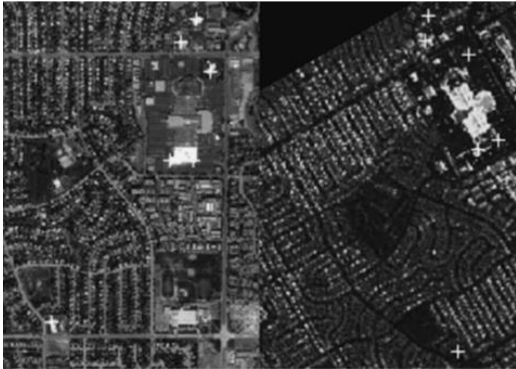
Figure 3: Final set of detected control points (as indicated by crosses). (Left) Optical image. (Right) LiDAR image. Note: This Figure shows the effectiveness of the methodology developed by Wong and Orchard [13] in control point detection. Courtesy: (Wong and Orchard 2008), IEEE transactions on Geoscience and Remote Sensing.
