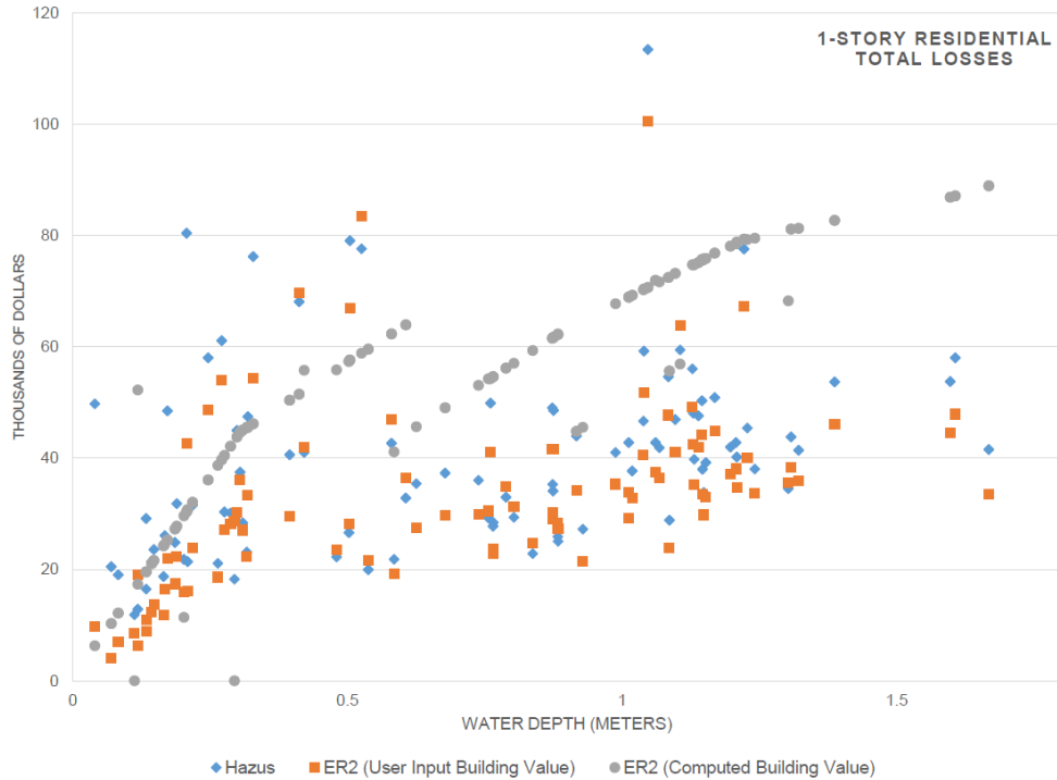
Figure 3.9 Total Damages versus water depth for Hazus, ER 2 using user input building value and ER 2 using computed building value
