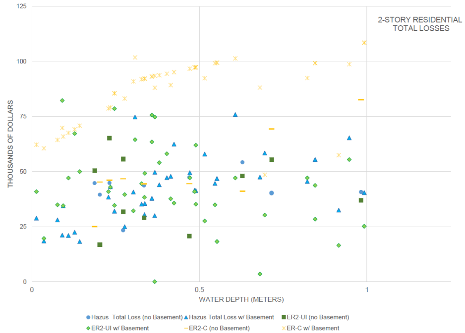
Figure 3.10 Total Damages versus water depth for Hazus, ER 2 using user input building value and ER 2 using computed building value, 2 Story residences, with and without basements
