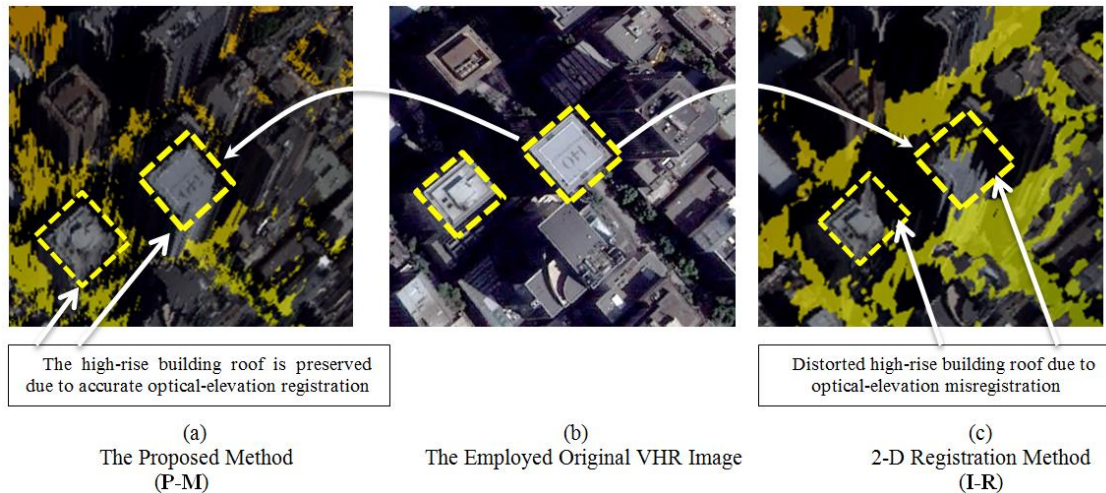
Figure 2.5 3D representation of the registration results achieved for a subset of the datasets used. (a) The registration result achieved by using the proposed method. (b) The original optical off-nadir imagery provided to show the level of distortion. (c) The registration result achieved by using 2 nd order 2D polynomial. The yellow color surface represents the terrain (thresholding surface) and hence objects above this surface represent building hypotheses generated in the scene.
