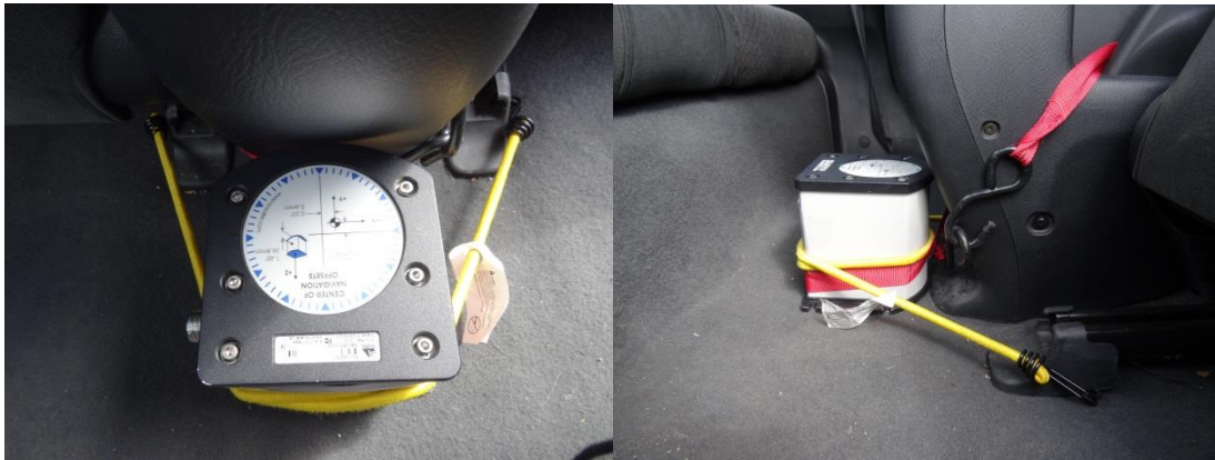
Figure 5-1: IMU-LN200 strapped to vehicle
