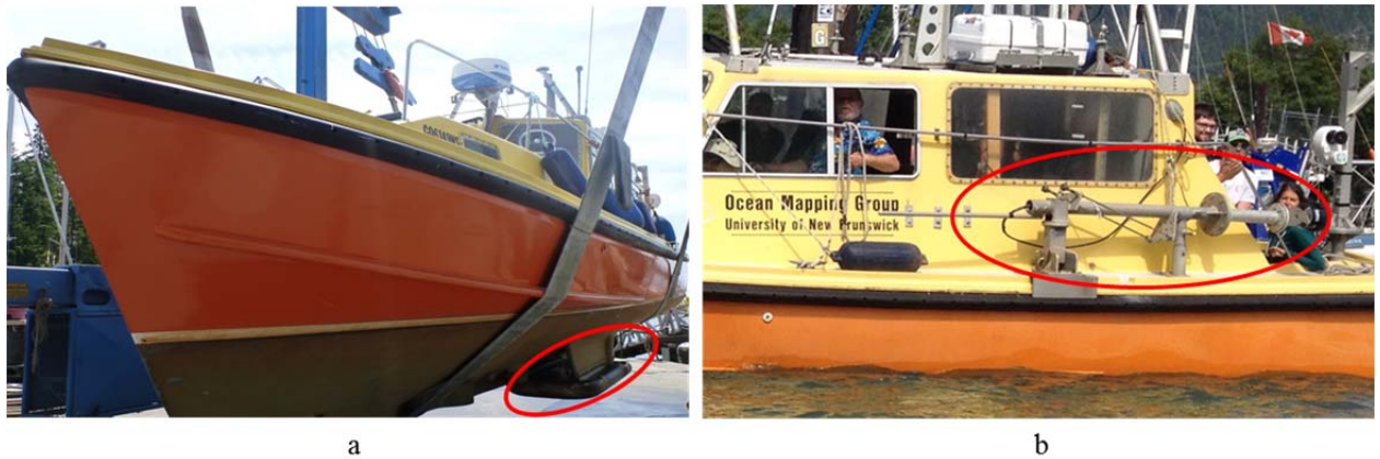
Figure 3.7: A gondola on the Heron where the EM710 is mounted (a) and retractable mount pole for the M3 (b).
