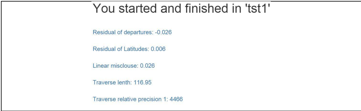
Figure 0.11: students will access this information when they are using the tool by themselves. The residuals, linear misclosure and traverse length are in meters.
