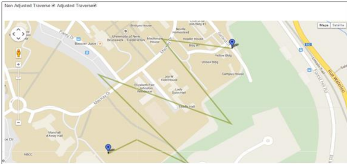
Figure 0.8: this figure shows the first type of traverse, which starts in a point and finishes in a different one. The traverse data shown in this figure was generated synthetically with a Matlab script.
