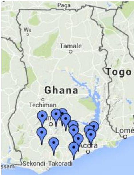
Figure 4-19 Location of trigonometric levelling stations Source of map: Google
