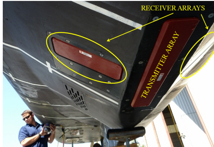
Figure 2.10: Example of an EM 2040D transducers installation (after Hughes Clarke et al. , 2013)
