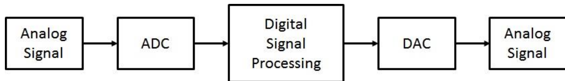
Figure 3-- Typical Digital Signal Processing System Diagram
