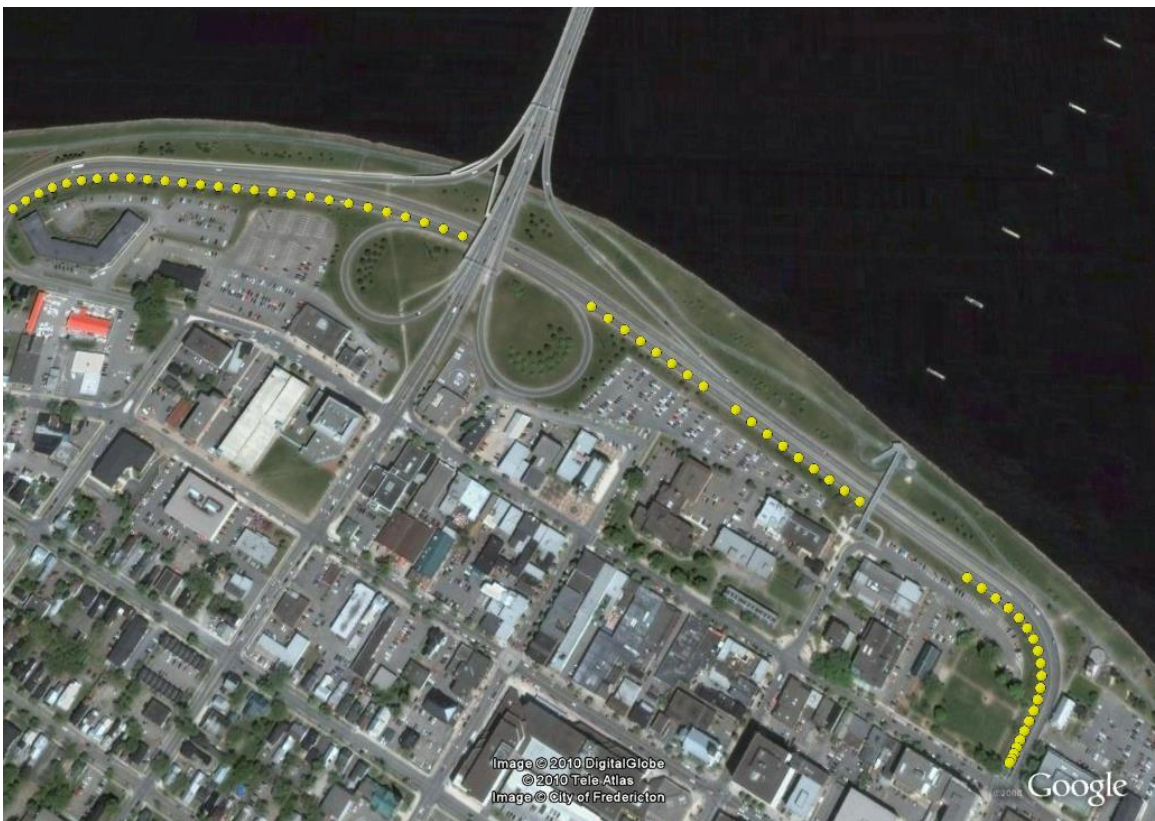
Figure 2.4: Car trajectory in Fredericton, New Brunswick, Canada. The receiver lost lock twice on all satellites due to overpasses. (Imagery courtesy of Google.)
