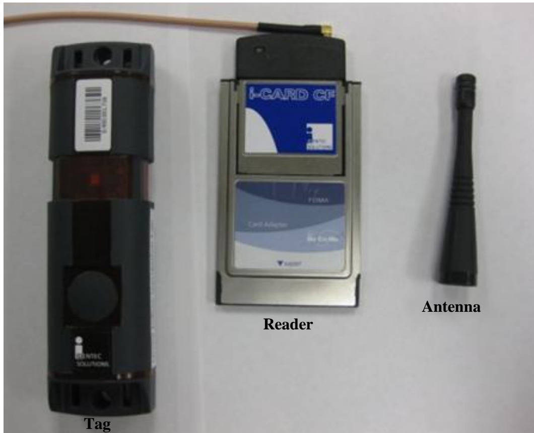
Figure 5.6 RFID system components.
