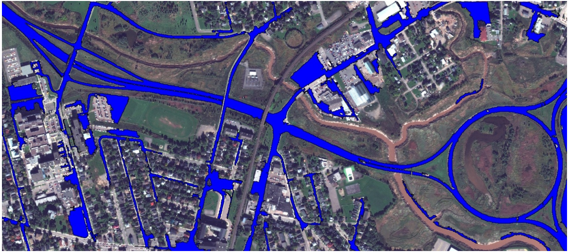
Figure 5.5 The result of the proposed object-based road extraction overlaid on the Pan-sharpened image. The extracted roads are the blue areas.
