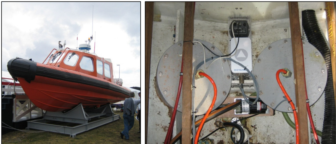
Figure 3.1 - One of the survey launches of the Dutch Navy (left). Top view of the EM3002 dual head system, with the motion sensor (OCTANS) in the middle (right).
