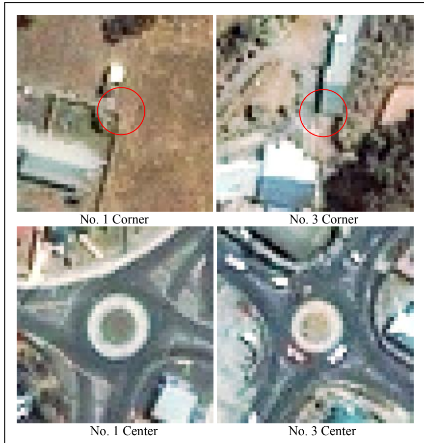
Figure 2.22 Samples of Corners and Centers. The corner is very blurry, while the center is clear.
