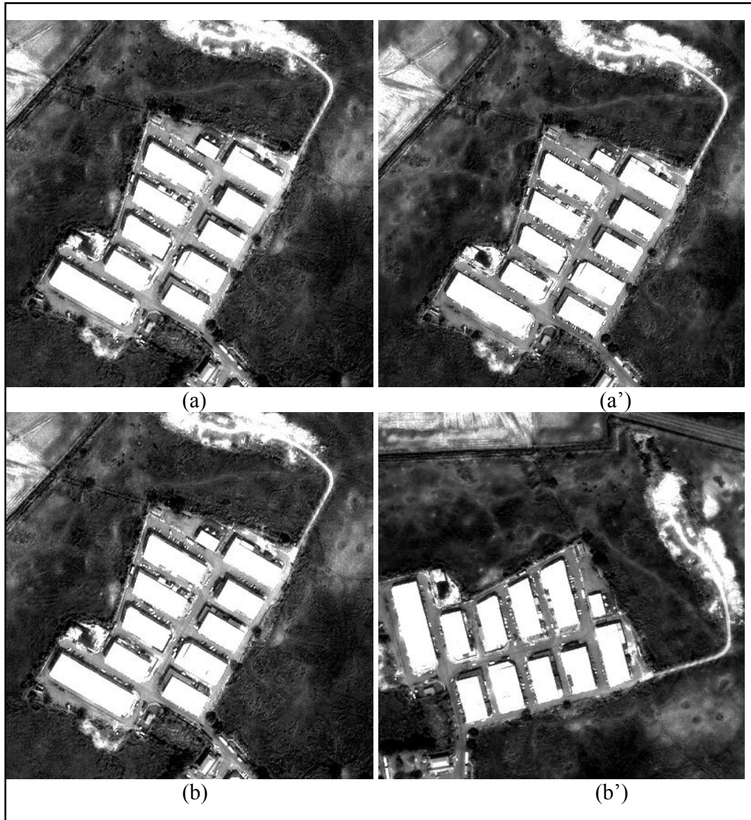
Figure 3.12 Test Images From the Penang Stereo Pair: (a) and (a') are a pair (400 by 400 pixels) without rotation, while (b) and (b') are a pair (400 by 400 pixels) with (b') rotated 45°.
