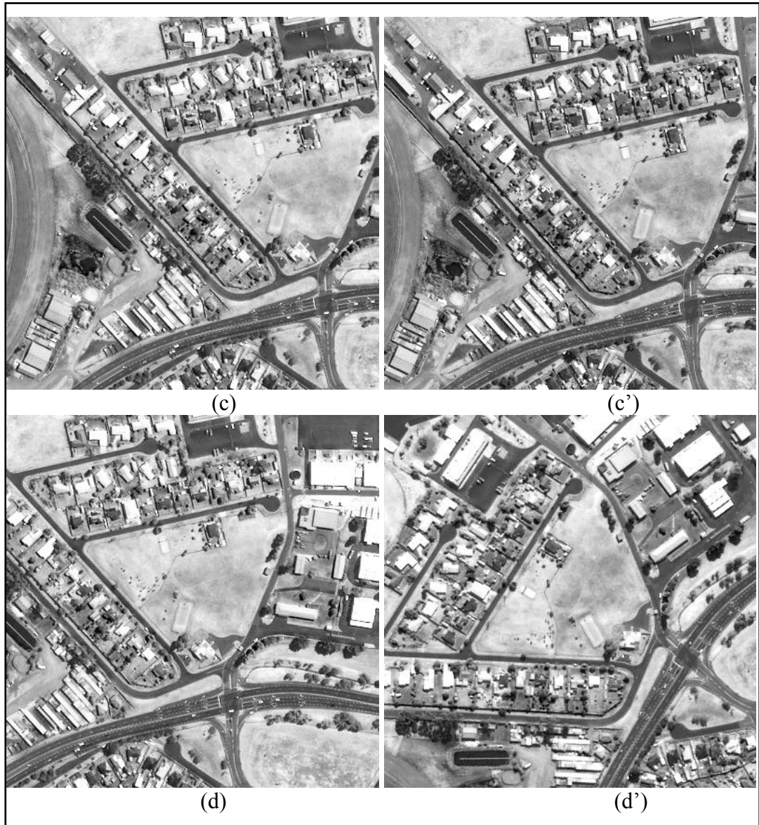
Figure 3.15 Test Images From the Hobart Stereo Pair: (c) and (c') are a test image pair (400 by 400 pixels) without rotation, and (d) and (d') are a test image pair (400 by 400 pixels) with (d') rotated 315°.
