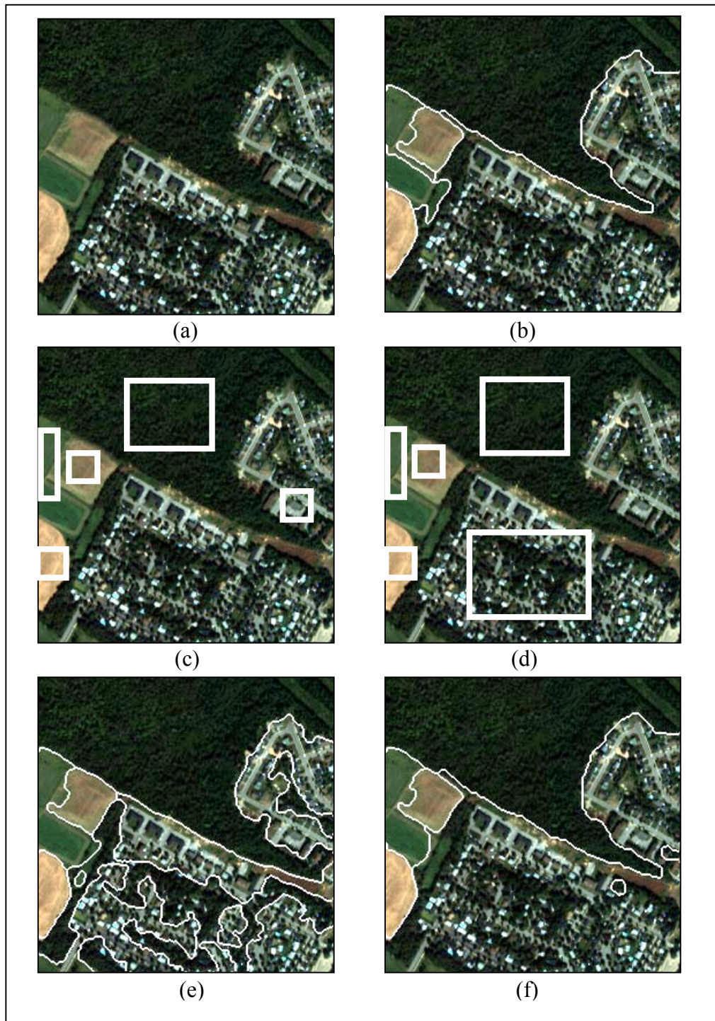
Figure 6.5: Supervised Segmentation. (a) test image; (b) unsupervised result; (c) large scale (more detail) templates; (d) small scale (less detail) templates; (e) result using large scale templates; and (f) result using small scale templates.
