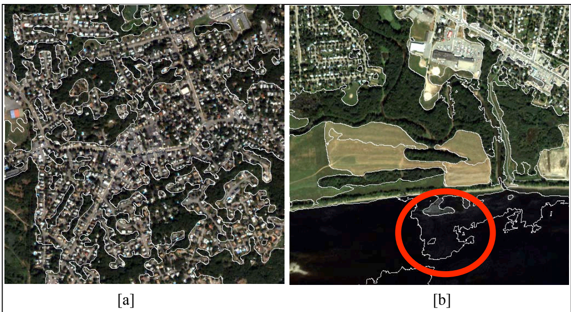
Figure 1.4: Example of segmentation inconsistency using the same segmentation methodology with a static set of parameters. [a] successful segmentation of land coverage in a suburban Boston, USA scene, and [b] unsuccessful (over) segmentation of land coverage in the city of Fredericton, NB Canada.
