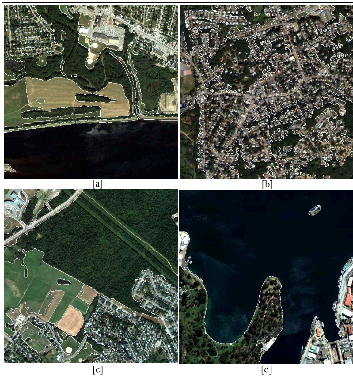
Figure 2.9: Automatic segmentation of QuickBird 2.44m multi-spectral imagery using the proposed FBR HSMR with generic algorithm modifications.
