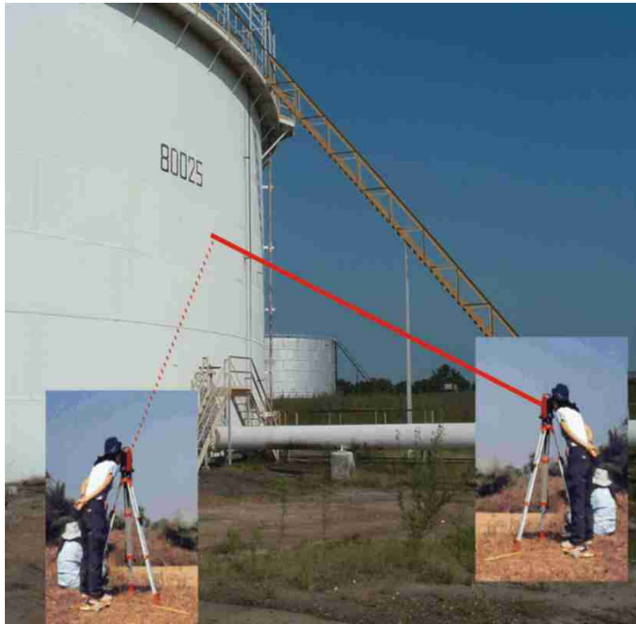
Figure 4.5 Surface tank measurements by intersection of angles (simulated)
