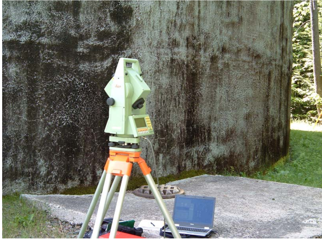
Figure 6.2 ALERT SCAN and the RL RTS collecting data of the water tank
