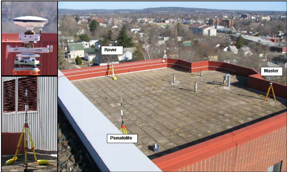
Figure 6.12: Displacement Detection Experiment Configuration (Top Left: Rover Antenna on Translation Stage, Bottom Left: IN200 Pseudolite, Right: Observed Baseline).
