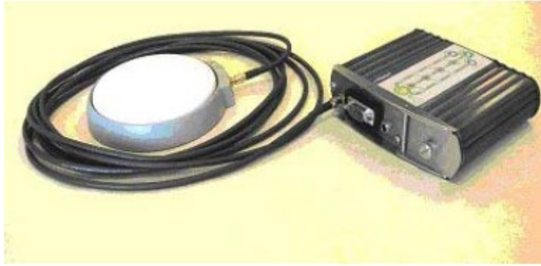
Figure 4.2.4 – A CDGPS Receiver which receives modified RTCA corrections and converts them to RTCM v2.3 corrections. [CDGPS, 2003].
