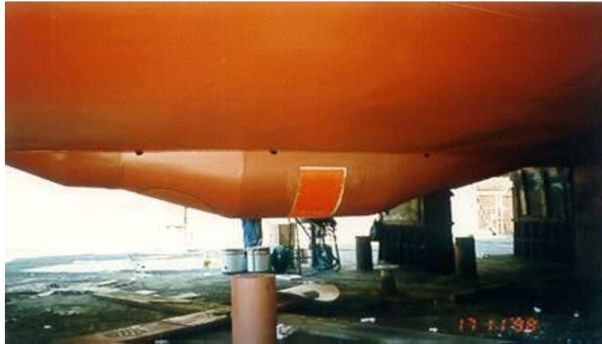
Figure 2.2 EM1000 transducer installed in a fixed-mounted way in the prominent structure (0.5 m height) at the keel of the Hydrographic Ship Taurus.
