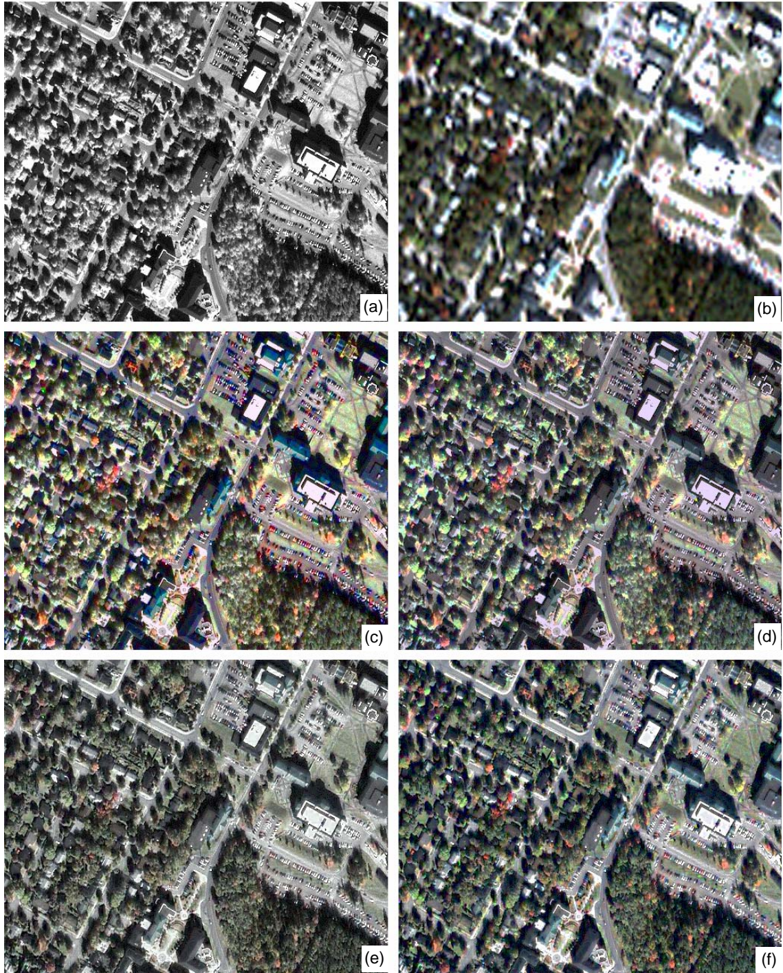
Figure 2.4. IKONOS image in Fredericton, Canada, and different fusion results ( 256 \times 200 pixel subset) (a) Original panchromatic image; (b) Original multispectral image with bands 1, 2, and 3; (c) IHS fusion result with the cylindrical model; (d) IHS fusion result with the triangular model; (e) Wavelet fusion result; (f) Result of the proposed IHS and wavelet integrated method.
