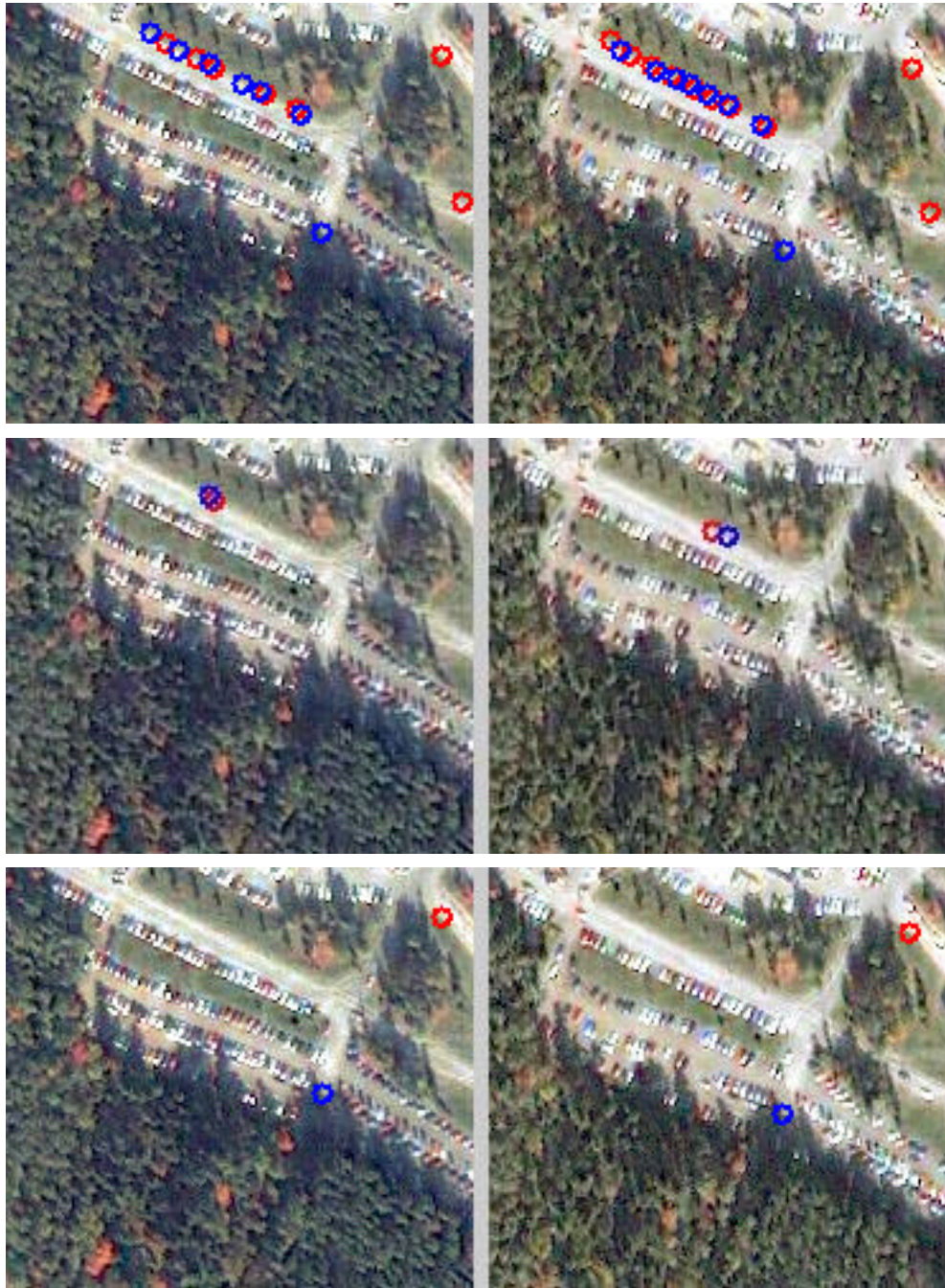
Figure 3-15. Automatically locating the best match in a tiled stereo image pair.
