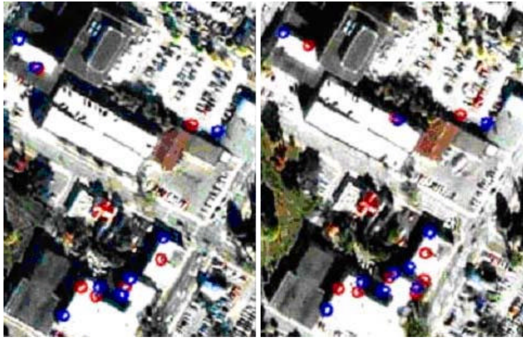
Figure 3-14. Results of searching for candidate matches Blue or red circle pairs correspond to maxima or minima matches, respectively.
