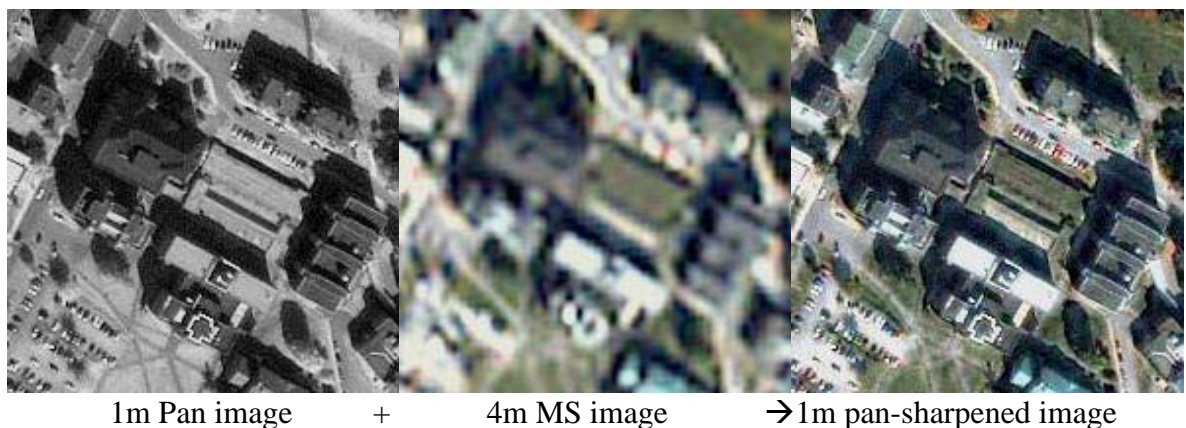
Figure 3-2. An example of pan-sharpened MS image generation (Location: UNB, Fredericton)
