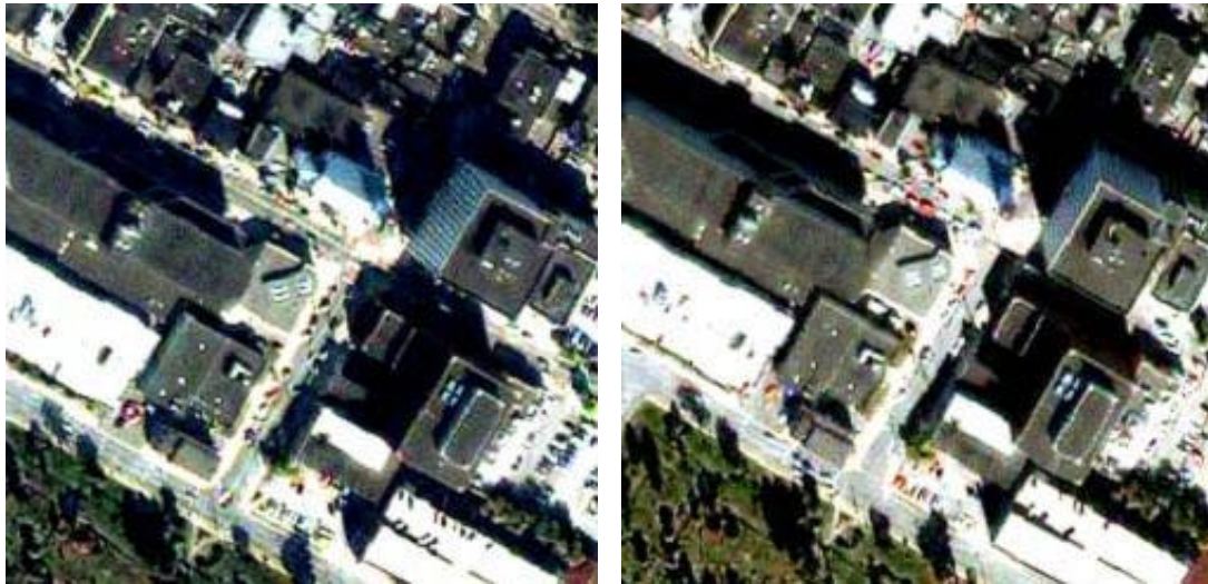
Figure 3-3. An example of pan-sharpened high-resolution MS satellite stereo images (Location: downtown Fredericton)
