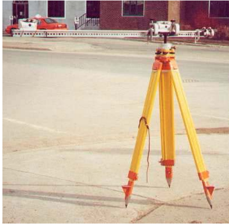
Figure 3.4. Left camera mount showing centre of rotation close to nodal point
