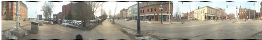
Figure 3.18. Seamless output mosaic as the product of automatic warping, alignment, blend, and end-to-end alignment for City Hall, Fredericton, NB, test location
