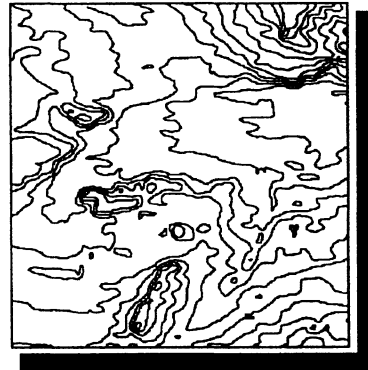
Figure 3-3. Contours generated from filtered DTM (after Russell et al.[1995]).
