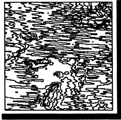
Figure 3-2. Contours generated from DTM containing ridging (after Russell et al.[1995]).
