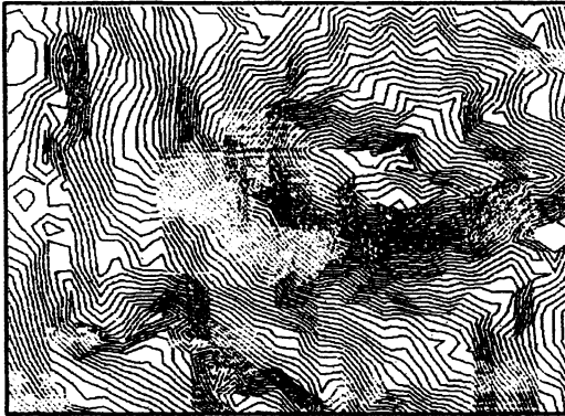
Image A: Contours generated from a TIN that is "Contaminated" with Ridging.
