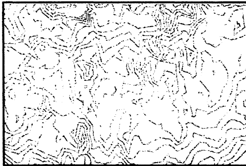
Image B: Contours generated from a randomly densified TIN.
