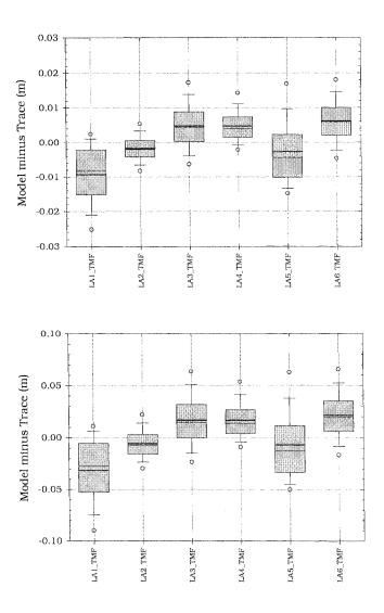
Figure 6.15 – Box-and-whisker plot for the differences between the different versions of the Lanyi mapping function and ray tracing (models minus trace), for  $10^{\circ}$  and  $6^{\circ}$  elevation angle.
