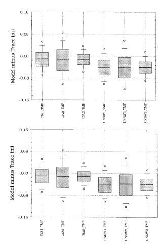
Figure 6.12 – Box-and-whisker plot for the differences between the different versions of CfA and UNSW mapping functions and ray tracing (models minus trace), for  $10^{\circ}$  (top) and  $6^{\circ}$  (bottom) elevation angles.
