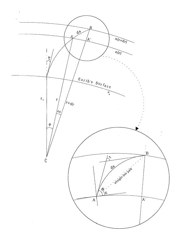
Figure I.1 – The ray trace geometry
