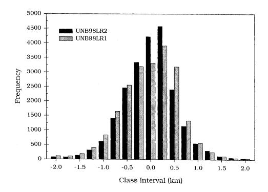
Figure 4.21 – Comparative histogram of residual distribution for UNB98LR1 and UNB98LR2, for a set of ~22,000 observations.
