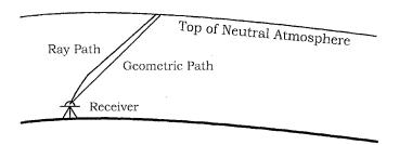
Figure 3.3 – The bending of the path of a radio wave. Due to variations in the refractive index, the ray follows a curved path.
