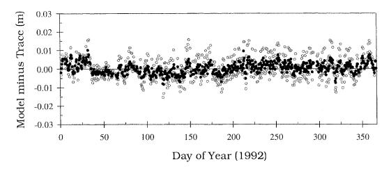
Figure 6.17 – Residual differences (model minus trace) for the LA6\_TMF with UNB98TH1 and UNB98LR1 driven by the instantaneous surface temperature (gray open circles) and driven by the mean monthly values of temperature (black circles), for the station Denver, for 10° elevation angle.
