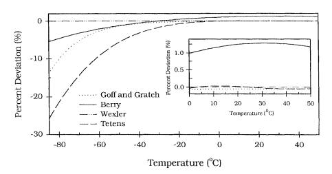
Figure 5.2 – Percent deviation for the Tetens, Berry and Goff and Gratch formulae as compared against the Wexler formula. All the formulae were extrapolated for temperatures below 0 °C. The error curves for temperatures above 0 °C are highlighted in the embedded plot.
