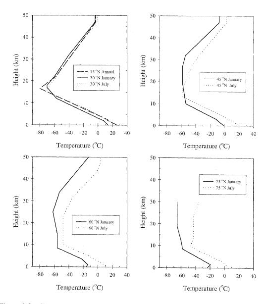
Figure 2.3 – Temperature profiles for the U.S. Standard Atmosphere Supplements, 1966, for the first 50 km.
