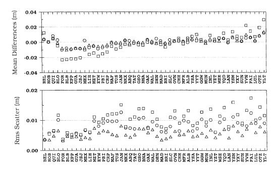
Figure 6.13 – Mean bias (top plot) and associated rms scatter (bottom plot) for CfA1\_TMF (circle), CfA2\_TMF (square), and CfA3\_TMF (triangle), at 10° elevation angle, for 50 radiosonde stations.
