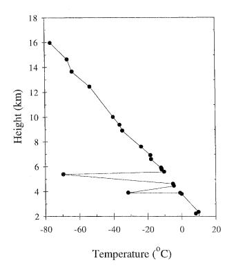
Figure 4.1 – Blunders in the temperature profile of a radiosonde sounding (sounding for Mexico City, January 30, 1992, 12<sup>h</sup> UTC, as given in the Radiosonde Data of North America (1946-1995) CD-ROM).
