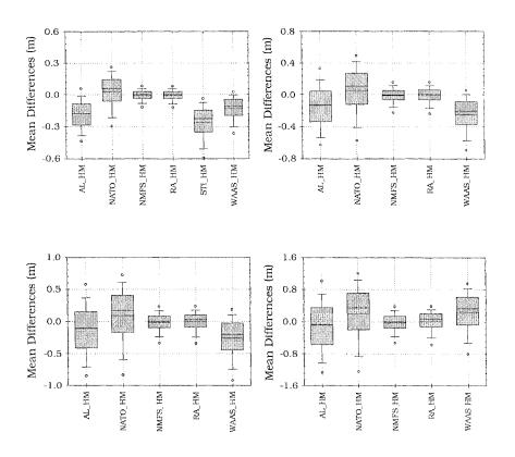
Figure 6.23 – Box-and-whisker plot for the differences between total delay hybrid models and ray tracing (model minus trace), for  $30^{\circ}$  (top left),  $15^{\circ}$  (top right),  $10^{\circ}$  (bottom left) and  $6^{\circ}$  (bottom right) elevation angles.
