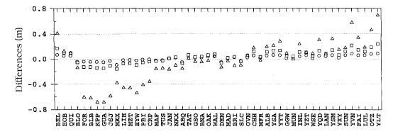
Figure 6.24 – Differences between the Rahnemoon and NMFS atmospheric models (Rahnemoon minus NMFS), at  $10^{\circ}$  (circles),  $6^{\circ}$  (squares) and  $3^{\circ}$  (triangles) elevation angles, for 50 radiosonde stations.
