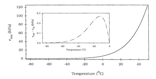
Figure 5.1 – Saturation vapor pressure over water ( $e_{sw}$ ) with extrapolation for temperatures below 0 °C, and the difference between the saturation vapor pressures over water (extrapolated) and over ice ( $e_{si}$ ). The computation of  $e_{sw}$  and  $e_{si}$  were performed using the Wexler [1976] and Wexler [1977] formulae, respectively.
