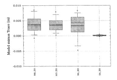
Figure 6.1 – Box-and-whisker plot for the differences between the zenith hydrostatic delay prediction models and ray tracing (model minus trace).
