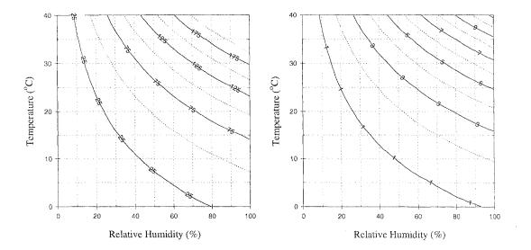
Figure 3.1 – Contour plots in refractivity units of the non-hydrostatic refractivity (left) and of the difference between the wet and the non-hydrostatic refractivities (right), for a wide range of temperature and relative humidity.
