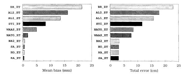
Figure 6.5 – Ranking of the zenith total delay models based on the absolute mean bias (left) and total error (right), for the total number of differences.
