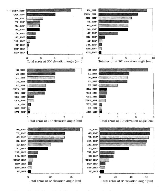
Figure 6.8 – Ranking of the hydrostatic mapping functions by total error.
