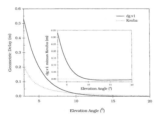
Figure 5.9 – Geometric delay prediction using dg.v1 and Kouba [1979].
