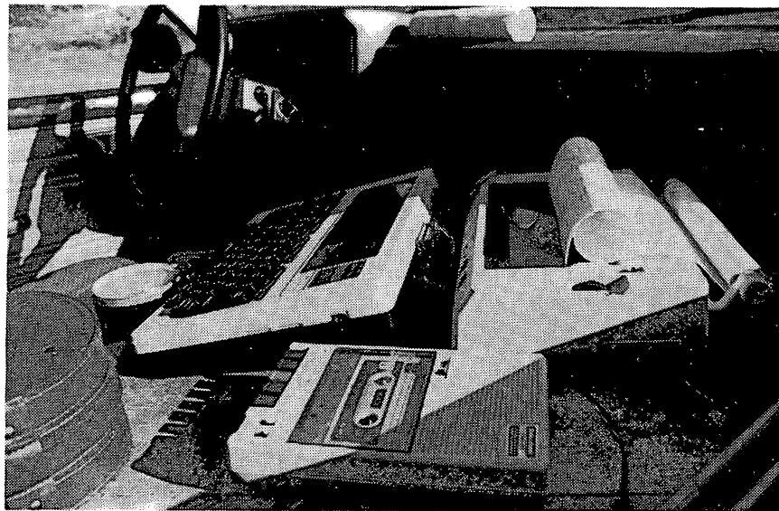
Fig. 26 TRS80 Model 100 with printer and cassette recorder mounted in the observing vehicle.
