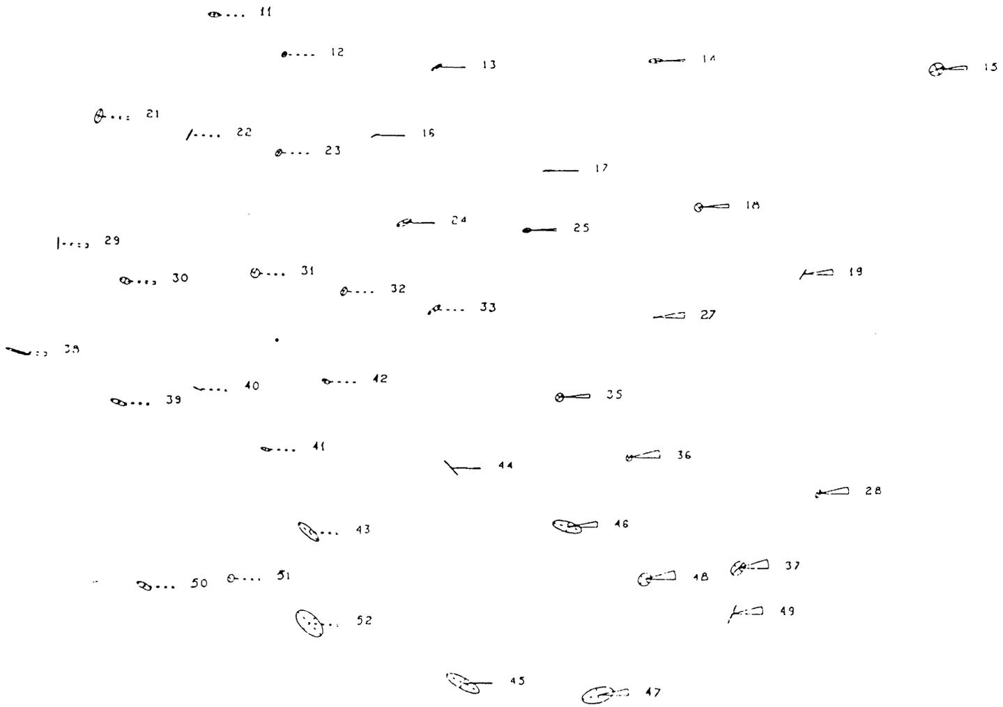
Figure 6.6: Strain induced in rigorous densification by the existing network (all points random errors only). Scale of strain ellipse axes: 1 cm = 7  $\mu$ strains. Scale of  $\omega$ , 1:1.
