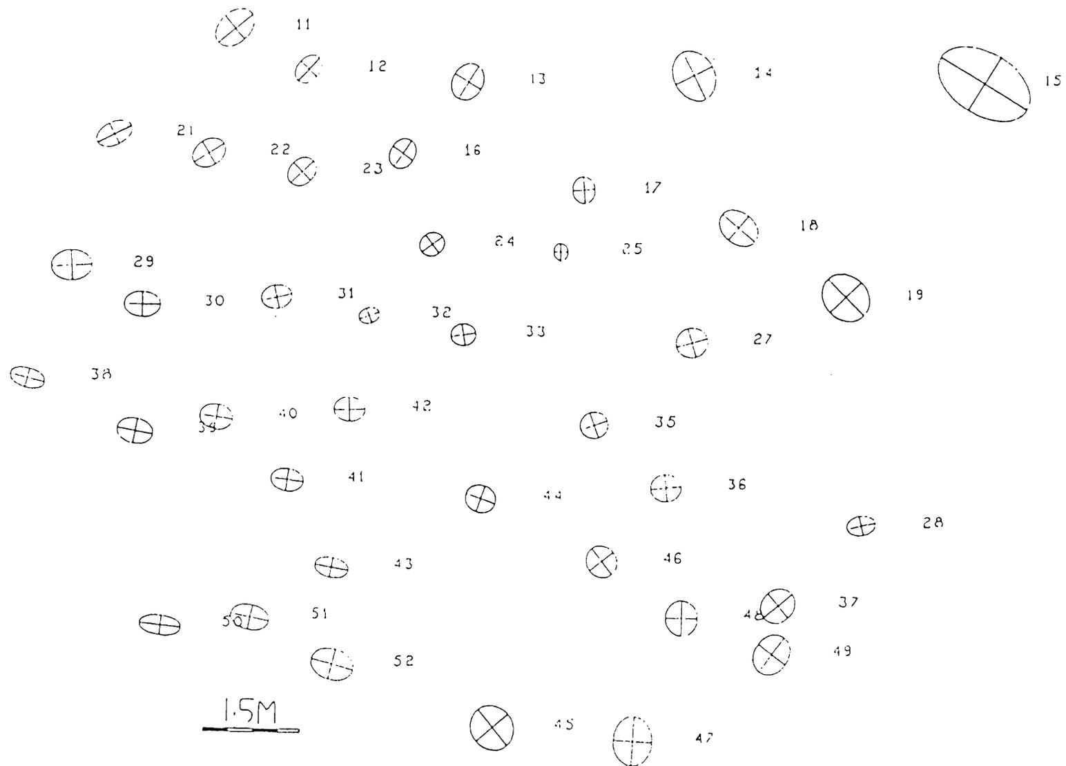
Figure 4-5: Absolute error ellipses in the rigorous densification at 95% confidence level.
