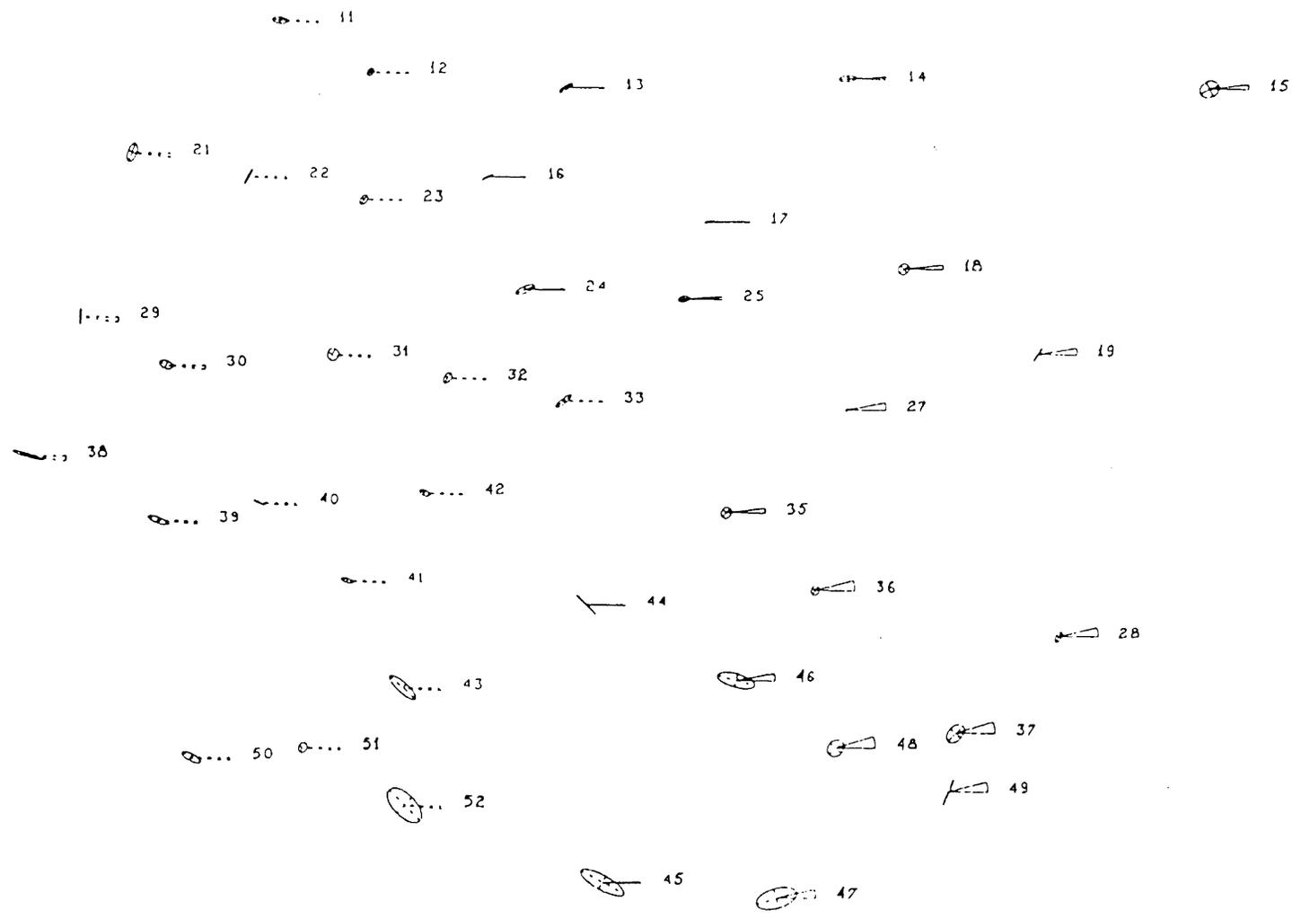
Figure 6.7: Strain induced in rigorous densification by the existing network (all points, random and biases). Scale of strain ellipse axes: 1 cm = 7  $\mu$ strain. Scale of  $\omega$ , 1:1.
