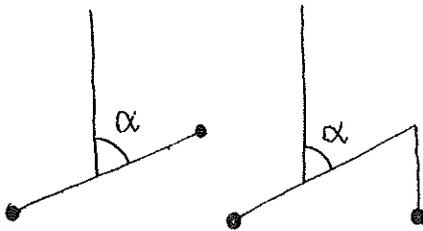
The inclination  $\alpha$  changes with the azimuth of the balance arm giving the values of gradients of  $g$  in various directions.
