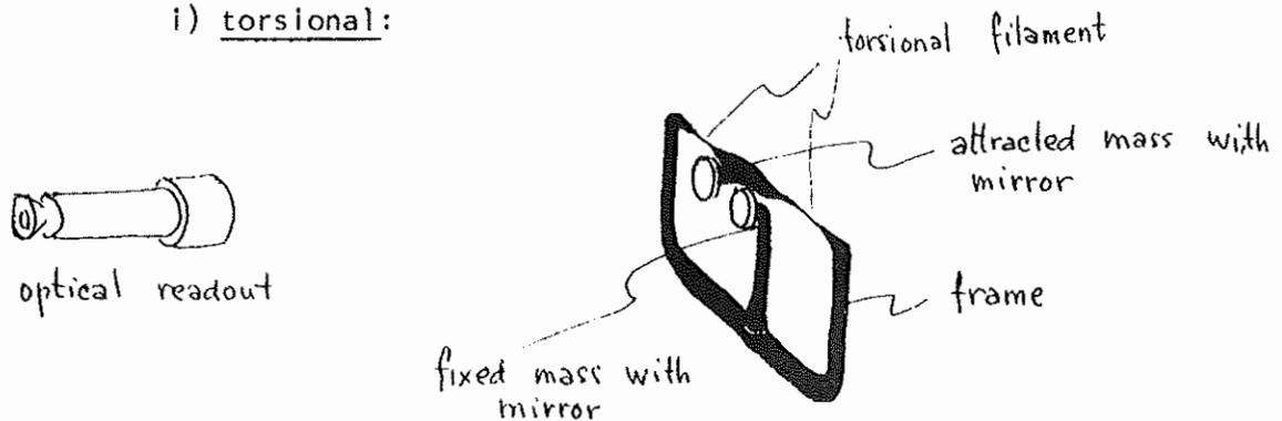
The whole construction is made of one piece of fused quartz. This design was first utilized in a Danish gravimeter designed by Norgaard (precision  $\pm 0.2$  mga). Basically the same design, although equipped with various compensational devices and different readout systems, is used by American Worden (precision  $\pm 0.03$  mgal) and German Graf gravimeters.
