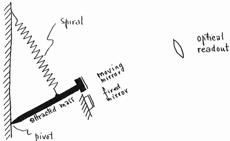
This system with various compensations and readouts is used by North American and Lacoste-Romberg (precision  $\pm 0.01$  mgal) gravimeters and seems to be the most successful one.
