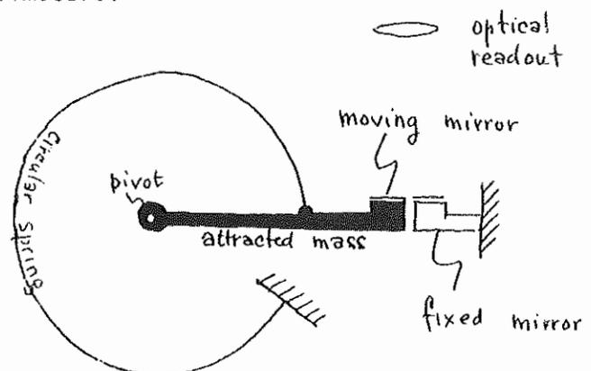
This is the principle used by Molodenskij in his GKA gravimeter (precision  $\pm 0.3$  mgal) and the whole family of subsequent Russian gravimeters. They vary by different compensational and readout system.
