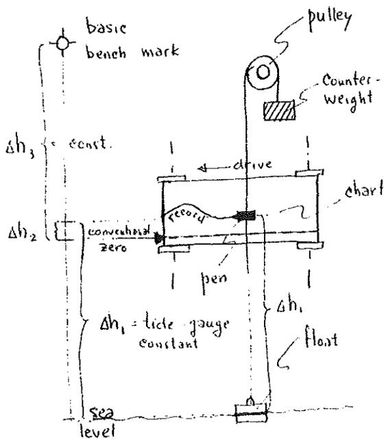
The levelling networks are usually connected to a number of basic bench-marks situated close to tide-gauges. Their heights (generally only a few meters above the sea-level) are determined as  $\Delta h_1 - \overline{\Delta h_2} + \Delta h_3$ , where  $\Delta h_1$  is a constant for a tide-gauge,  $\Delta h_3$  is the level difference between the tide-gauge zero and the bench mark and  $\overline{\Delta h_2}$  is the mean chart reading,
