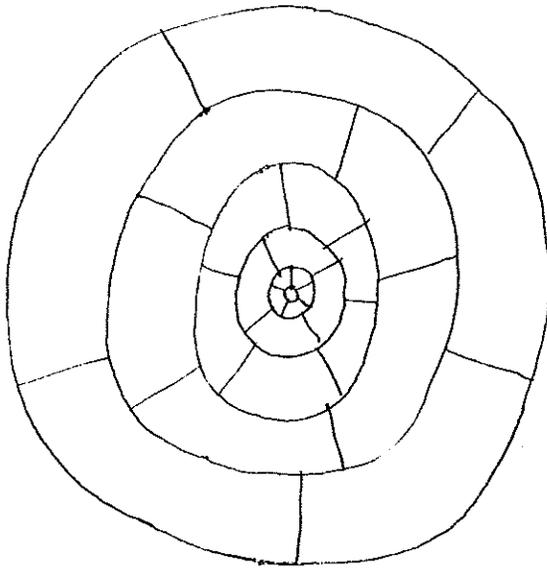
station into compartments according to a template. One of such possible divisions is shown on the diagram. The contribution of each individual compartment is computed separately and their combined effect then determined.
