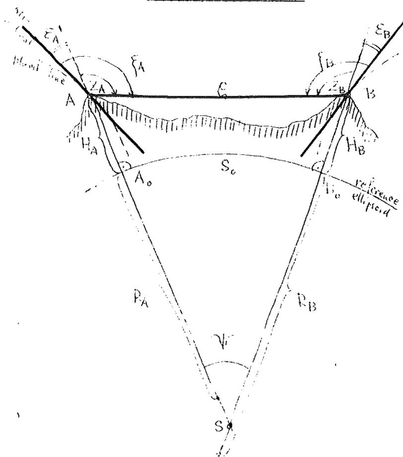
Leaving refraction aside, the zenith distances  $\zeta_A$ ,  $\zeta_B$  are what we get from the observations on the surface of the earth. On the other hand, the angles  $Z_A$ ,  $Z_B$  are the quantities we should like to get that would enable us to determine the difference in ellipsoidal heights of the two points A and B.
