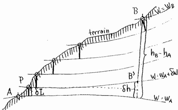
Let us consider a levelling line A,B with the intermediate stations depicted by circles. When we realize that the gravity field is represented by generally non-parallel equipotential surfaces, it is not difficult to see that the sum of the observed level
