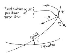
The forces acting on the satellite can be split into 2 parts: Ist due to the central field, 2nd, due to the disturbing field. As we have seen already, the first part does not cause any changes in the orbital elements  $\tilde{K}_{\alpha} \equiv (a, e, i, \Delta M, \omega, \Omega)$ . Only the disturbing
