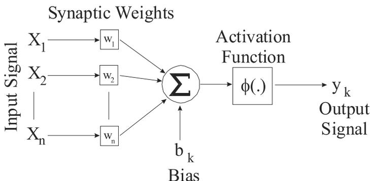
**Fig. 1.** Nonlinear artificial neuron model (adapted from *Haykin, 1999*).
