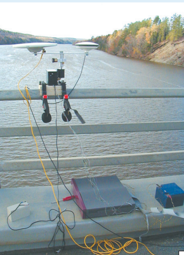
Figure 3 GPS antennas, reflector target and accelerometer housed together on the guardrail near the middle of the span
