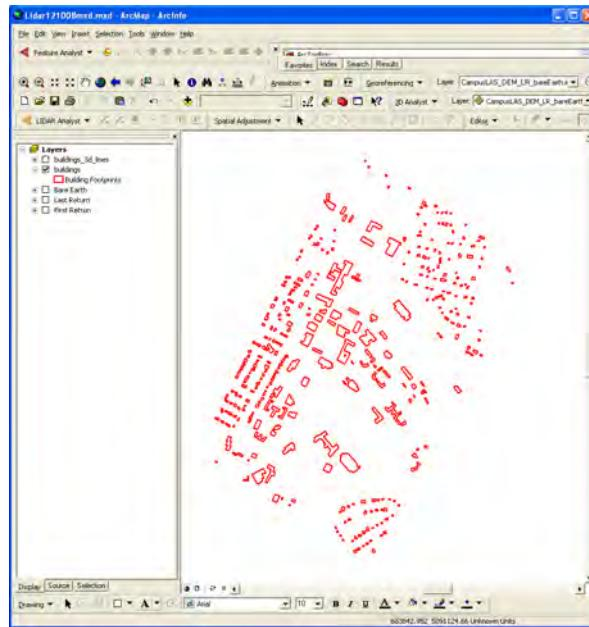
Fig. 9. Extracted Building polygons from LiDAR data
