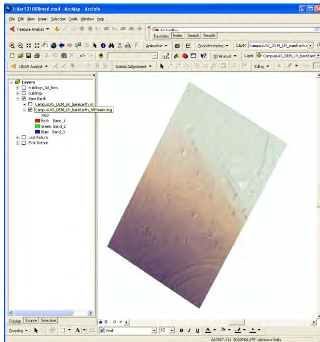
Fig. 8. Extracted ground surface from LiDAR data
