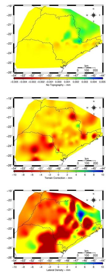
Figure 6: Corrections applied on Helmert's orthometric heights
