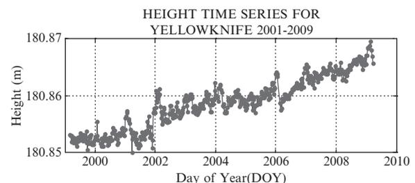
**Fig. 87.4** Height time series for the IGS station Yellowknife for the period of 1999–2009
