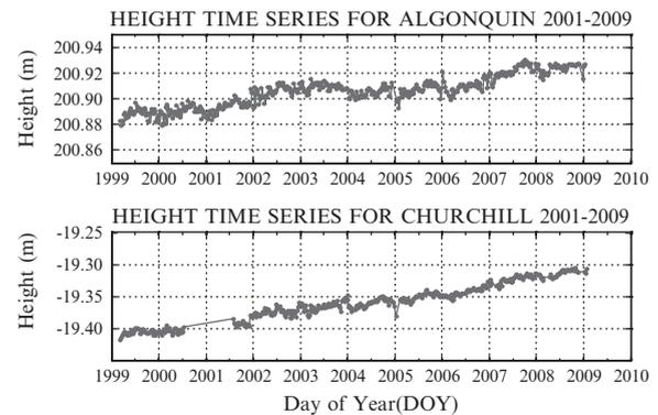
**Fig. 87.2** Height time series for the IGS stations Algonquin (*top*) and Churchill (*bottom*)
