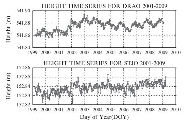
**Fig. 87.3** Height time series for the IGS stations DRAO (*top*) and STJO (*bottom*)
