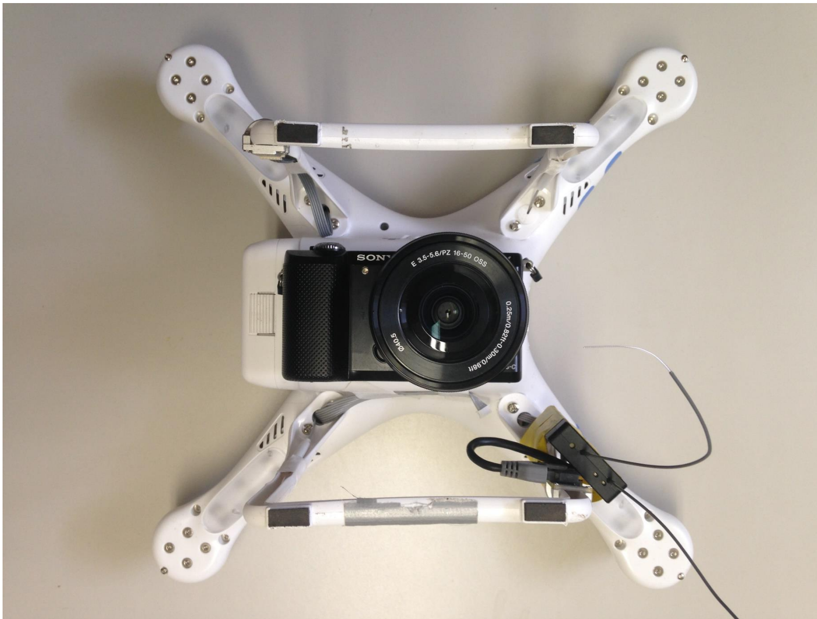
Bottom View of the Phantom 2 with Sony Alpha 5000 attached for vertical imaging (410g payload)
