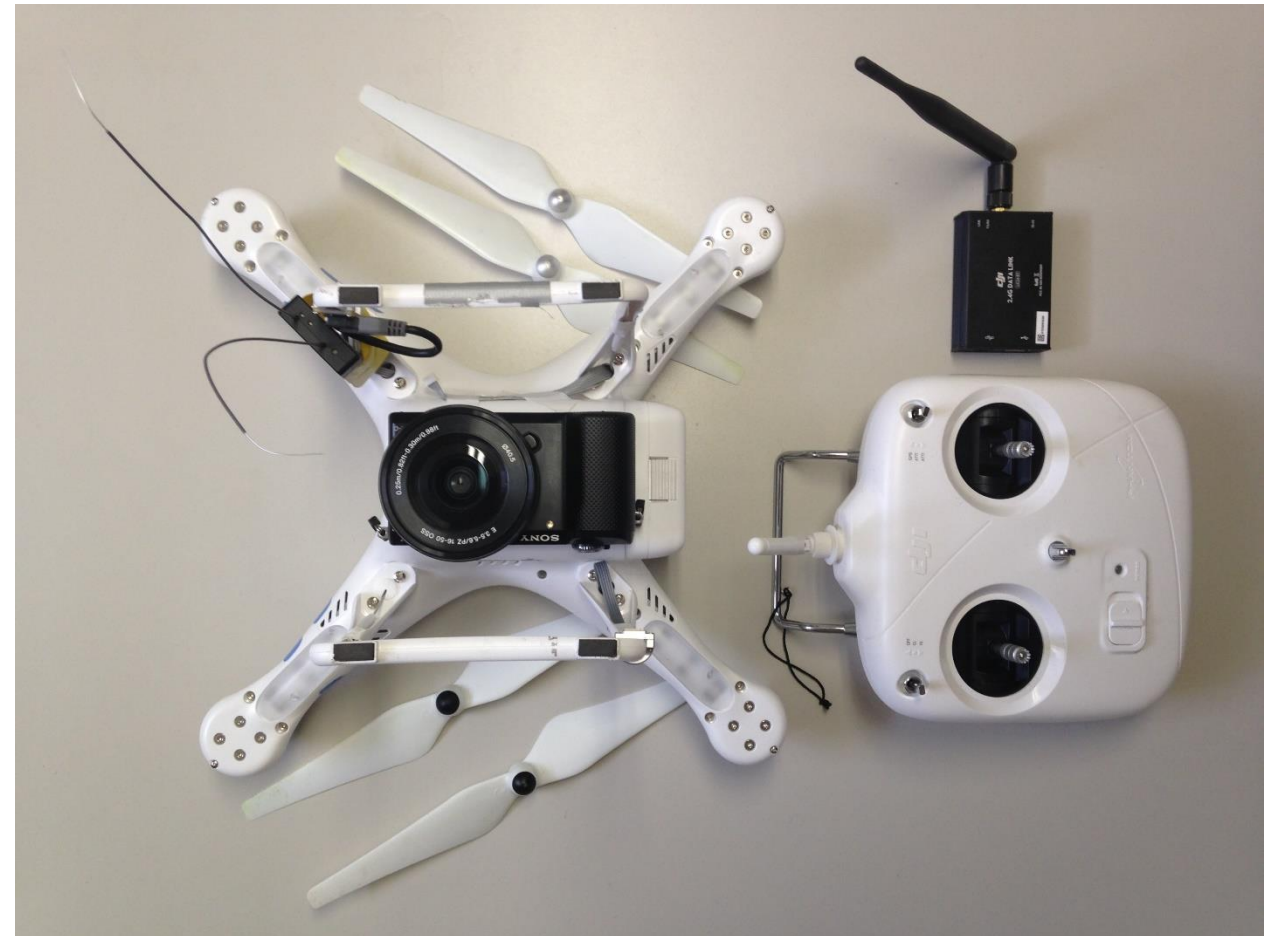
Left to right: Phantom 2, Sony a5000, 2.4G Bluetooth datalink, Controller
